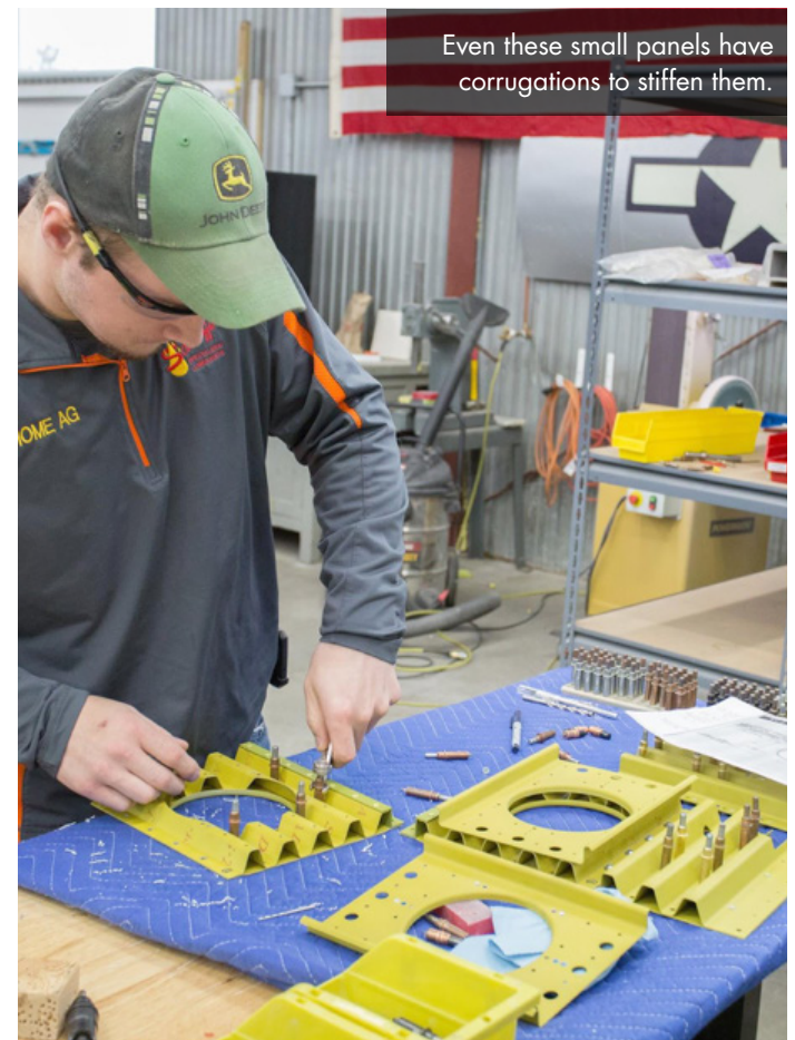
The pilot's floor is being fitted and this image shows the foot troughs clecoed in place. Many of the parts we have watched being fabricated, fit, and assembled had to come apart for paint.
