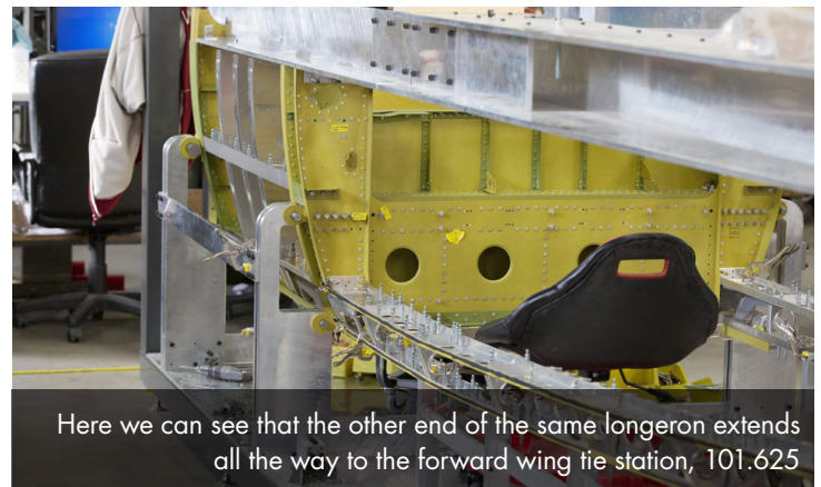
Notice the curve as the longeron sweeps upward toward the tail.
