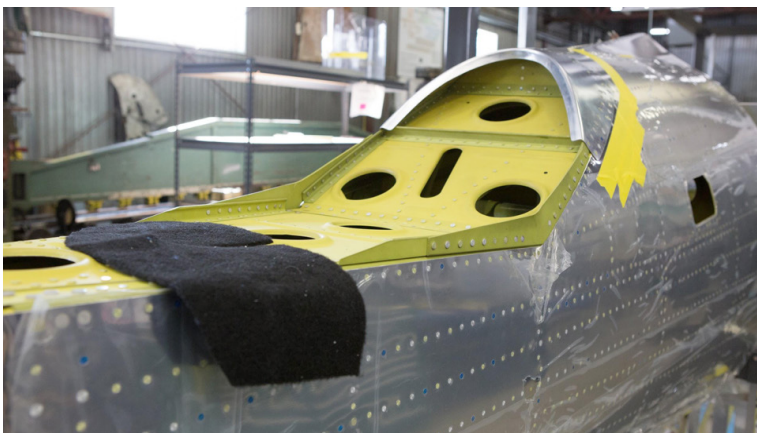
The mounting area for the horizontal stabilizer shows in detail in this closeup shot of the aft fuselage.
