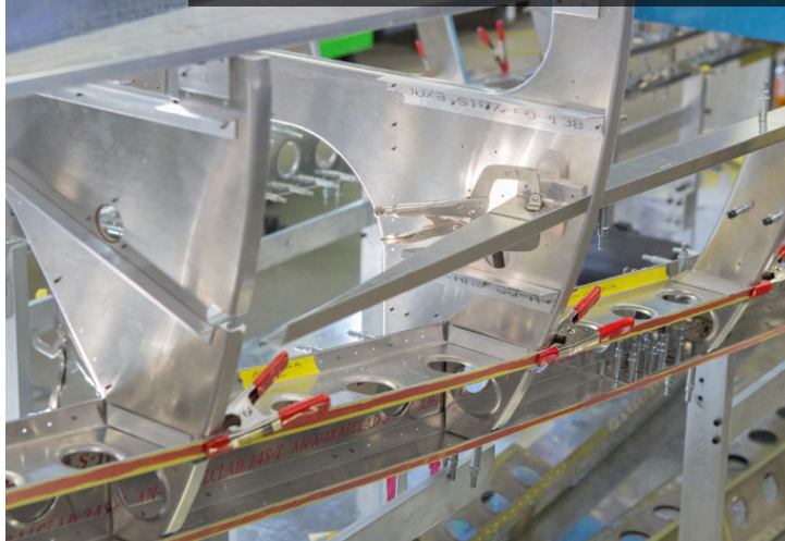
These fuselage formers are nearer the tail at station 285. Notice the stiffeners riveted to them.
