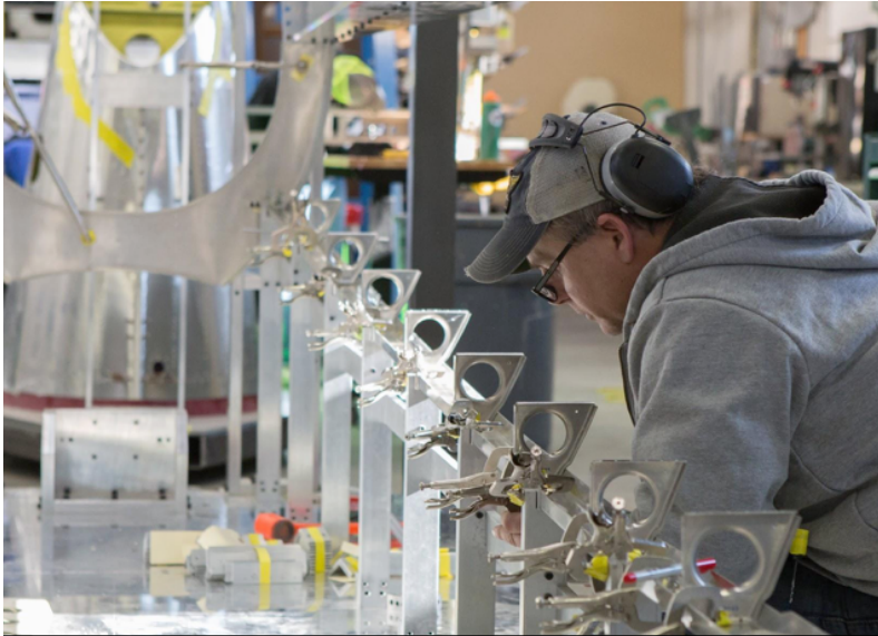
Robb checks the longeron. These lower longerons form a compound curve as they extend back and they each have over 30 separate pieces that need to fit perfectly to make the assembled longeron conform to the Thunderbolt's beautiful lines.
