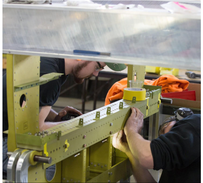
Hunter and Randy work on the now painted fuselage cross tie rib assembly. It is mounted in the fixture by the wing attach points.
