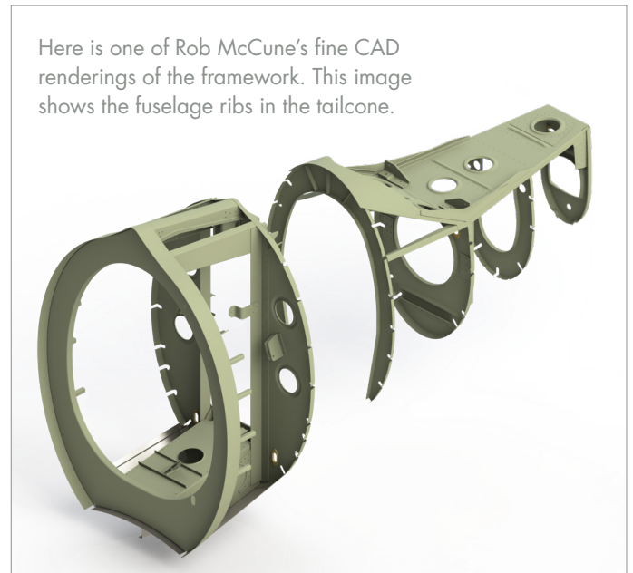
Here is one of Rob's renderings that was used for reference as the tail cone assembly was put together.
