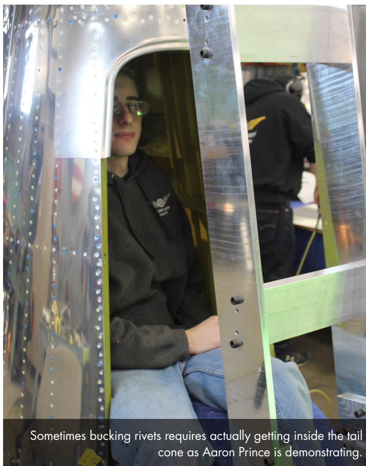
This shot shows the resulting aluminum skin after the entire template, cutting, and cleco fitting process has been completed.
