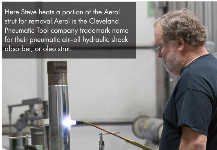
Steve Cotton is working on disassembly and initial inspection of the landing gear.
