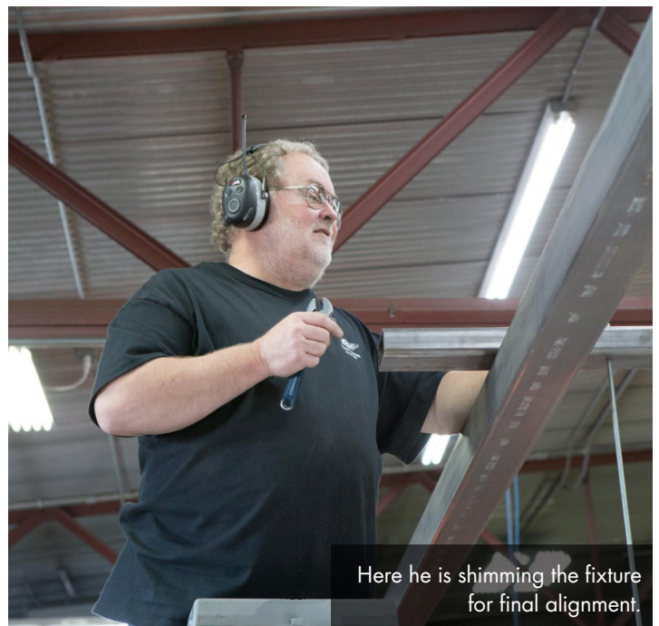
Steve checks the fixture for the forward fuselage for squareness and plumb.
