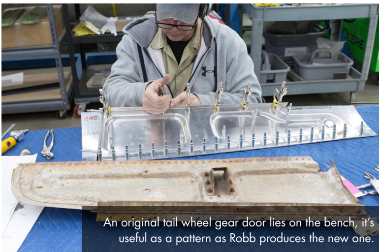
Randy works on skin for the rear of the tail wheel opening.
