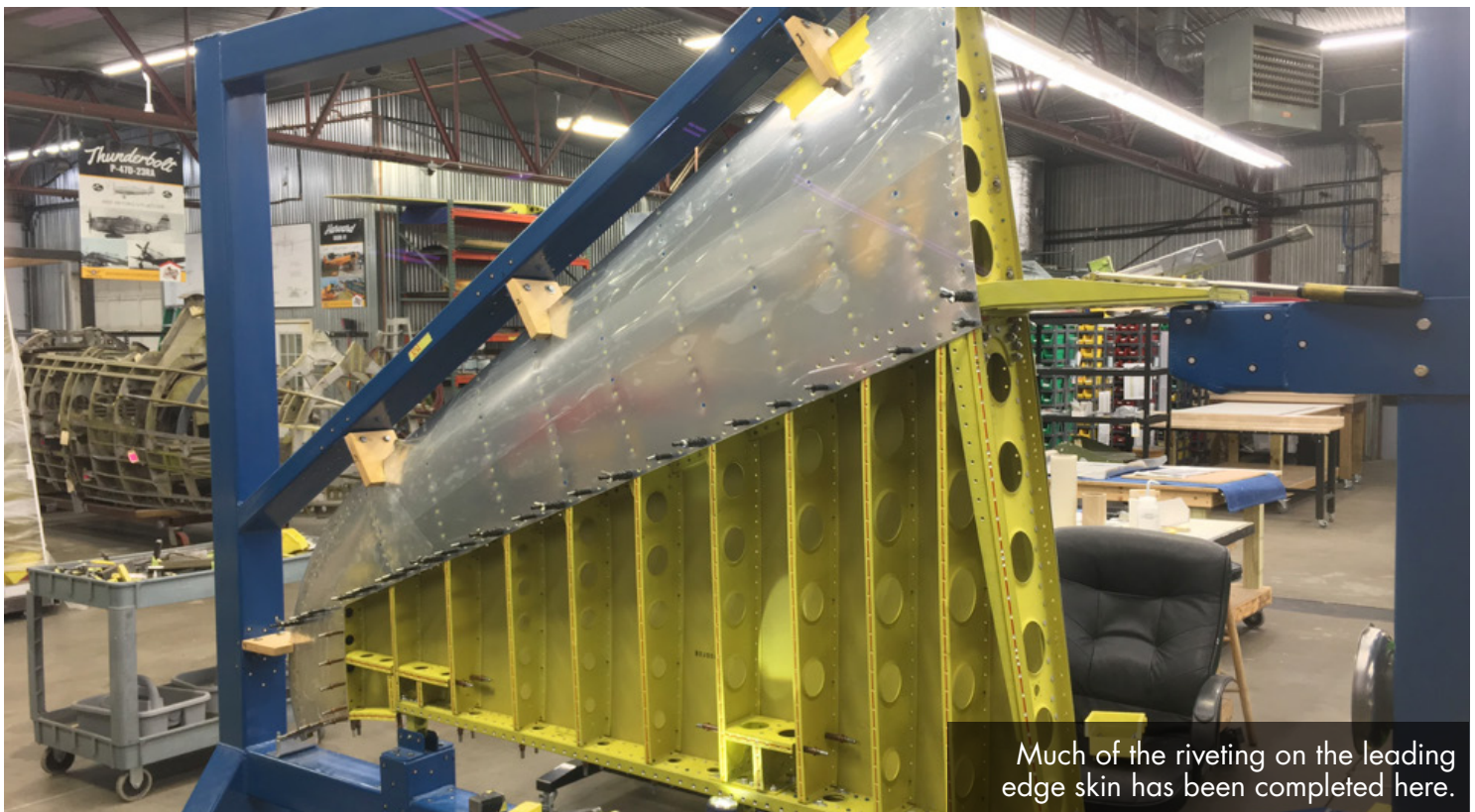
Randy works on fitting skin sections to the vertical stabilizer.
