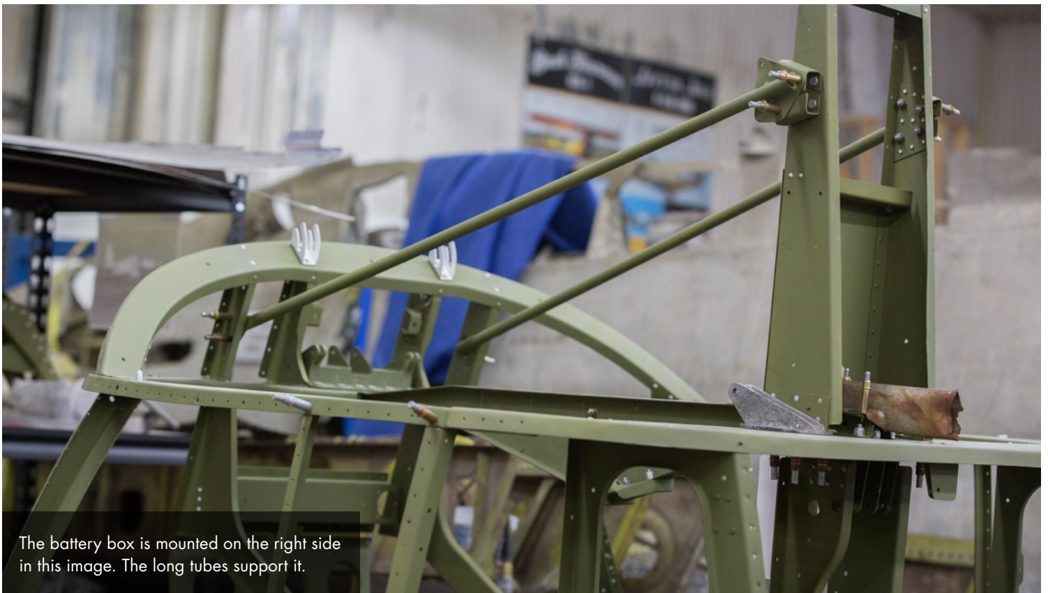
This structure is the instrument panel glare shield.
