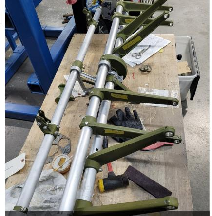
The two rudder pedal shafts and one of the brake pedal shafts are shown here. The eight painted arms are hangers that the rudder pedals mount on. The tube without pedal hangers is one of the brake tubes.
