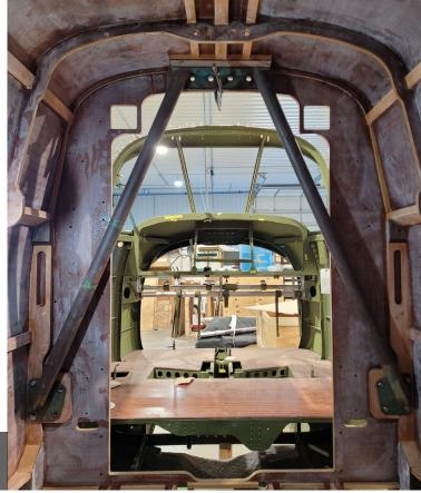
The metal forward fuselage as seen from inside the wooden rear fuselage
