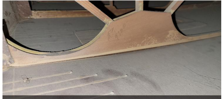
A look inside one of the NOS wings shows why it will have to be rebuilt. Even though these wings have never been used, some of the glue joints have delaminated over the 80 years since they were built.
