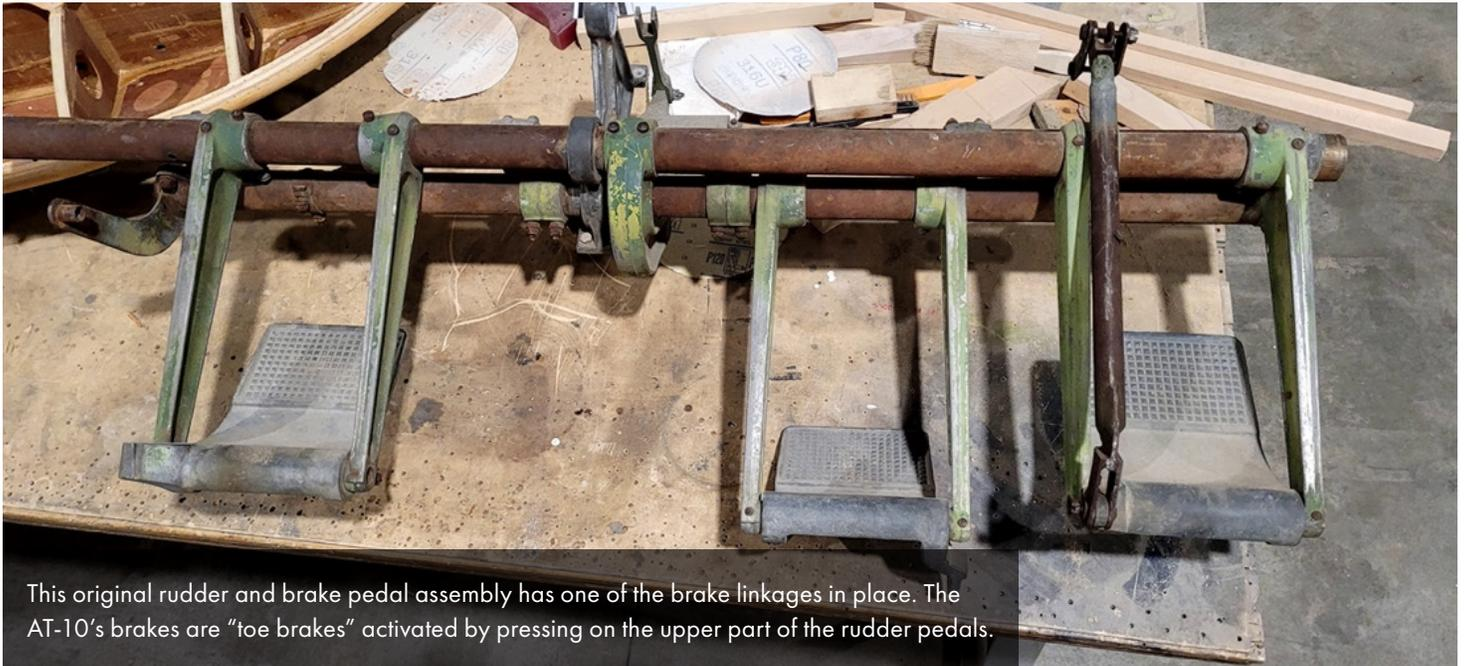
This original rudder and brake pedal assembly has one of the brake linkages in place. The AT-10's brakes are "toe brakes" activated by pressing on the upper part of the rudder pedals.
