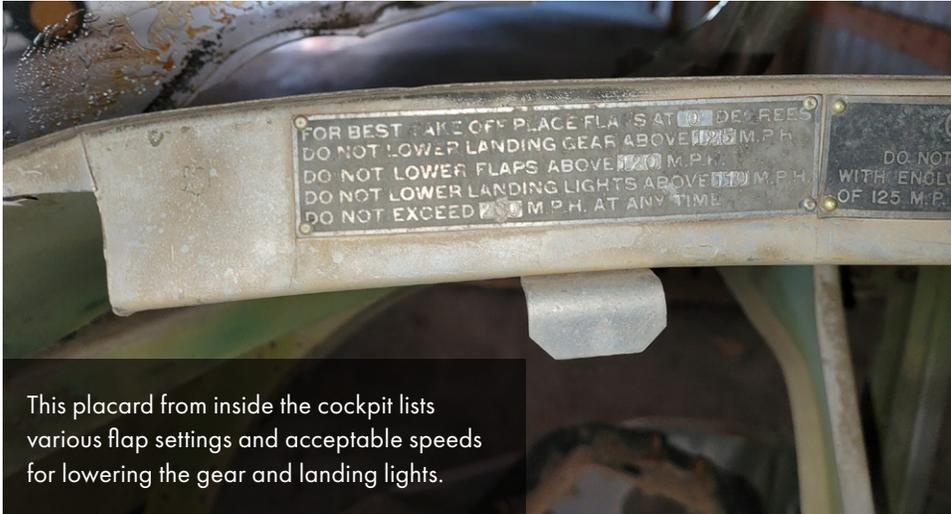
This placard from inside the cockpit lists various flap settings and acceptable speeds for lowering the gear and landing lights.
