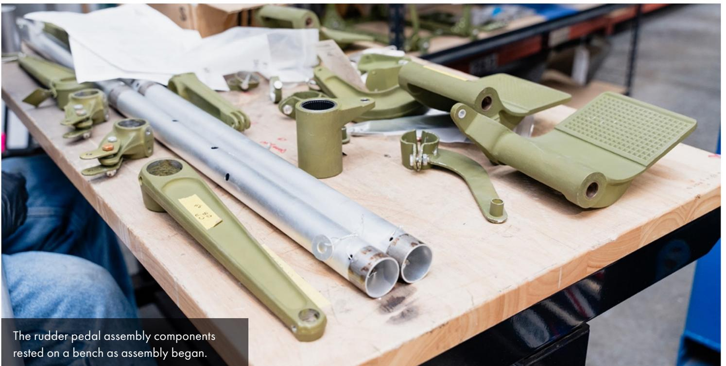
The rudder pedal assembly components rested on a bench as assembly began.
