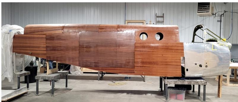
This is a side view of the fuselage with the cockpit area mated to the wood structure.
