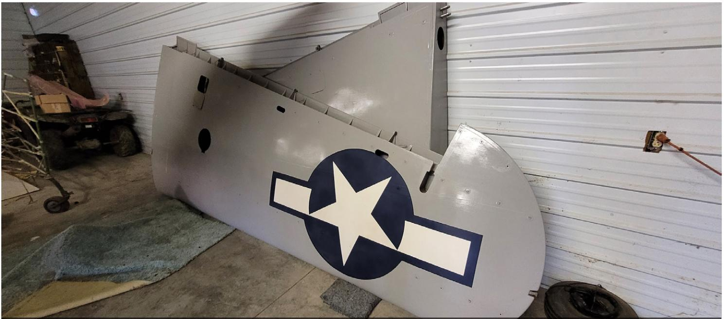
These are a set of NOS wings with the original fabric and dope finish in excellent condition. Not only is the finish original, but all the control pulleys and wiring inside the wing are in new, unused condition. Unfortunately, despite never having been used, the wings will still need to be rebuilt.
