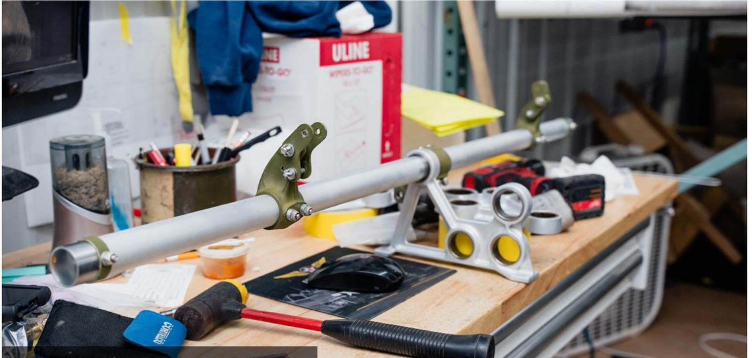
This shaft tube is one of four in the rudder pedal/brake pedal assembly. It is one of two tubes upon which brake linkages are mounted.
