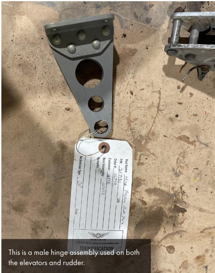
This is a male hinge assembly used on both the elevators and rudder.
