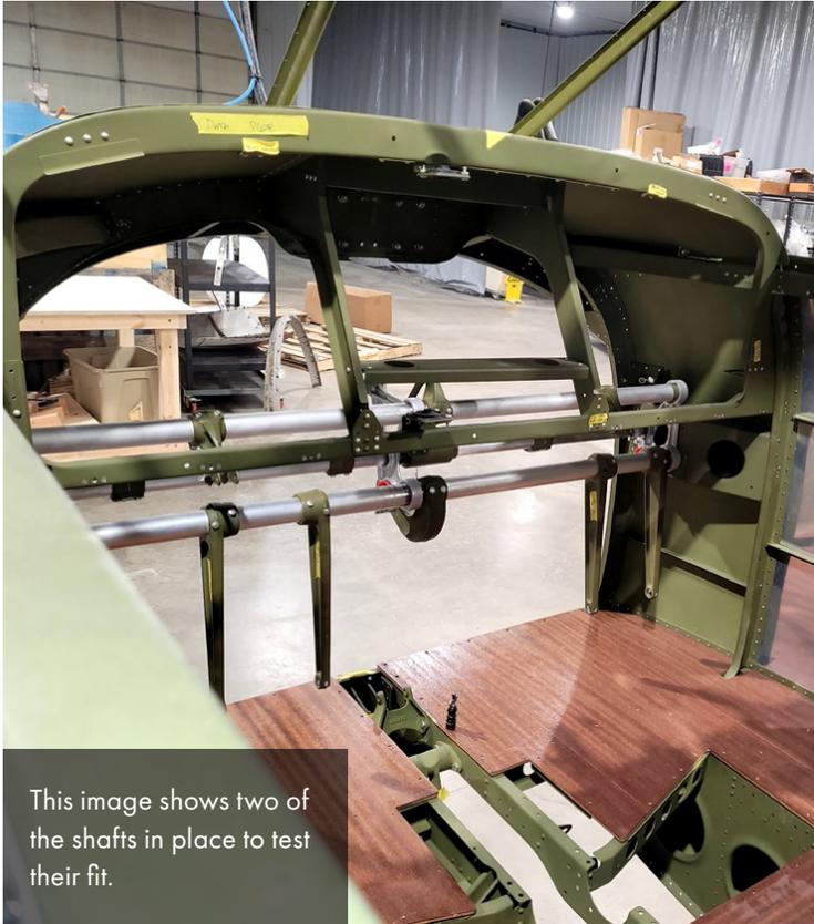
This image shows two of the shafts in place to test their fit.
