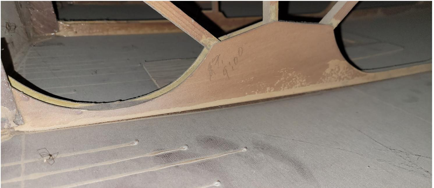
A look inside one of the NOS wings shows why it will have to be rebuilt. Even though these wings have never been used, some of the glue joints have delaminated over the 80 years since they were built.
