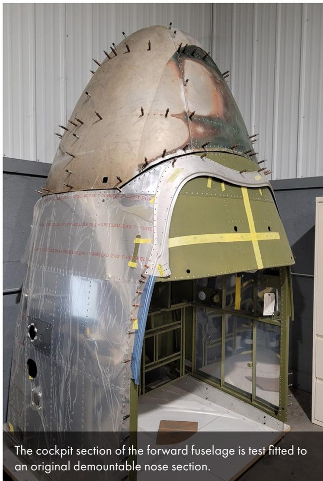
The cockpit section of the forward fuselage is test fitted to an original demountable nose section.
