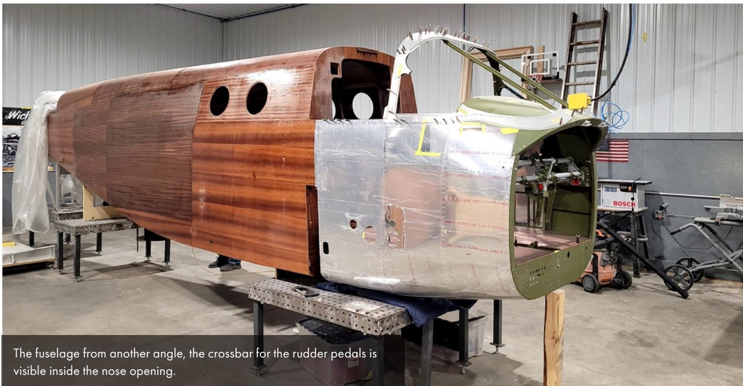
The fuselage from another angle, the crossbar for the rudder pedals is visible inside the nose opening.
