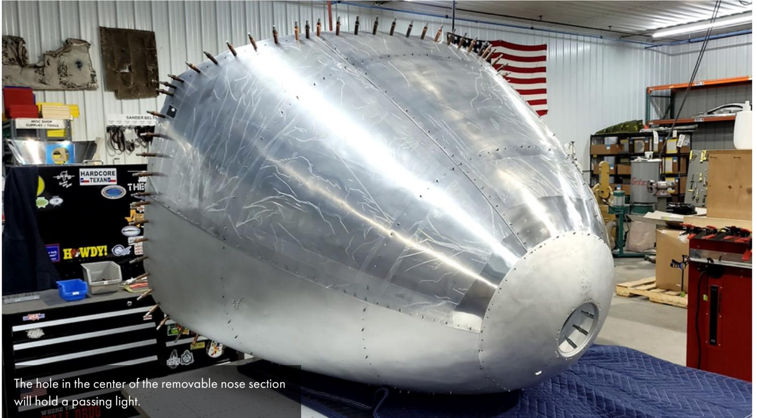
The hole in the center of the removable nose section will hold a passing light.
