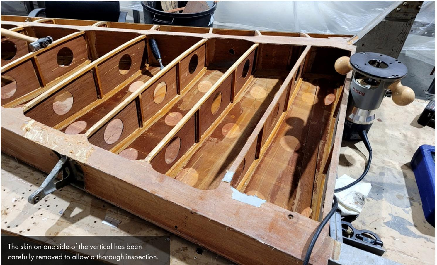
The skin on one side of the vertical has been carefully removed to allow a thorough inspection.
