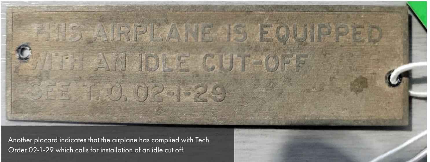
Another placard indicates that the airplane has complied with Tech Order 02-1-29 which calls for installation of an idle cut off.
