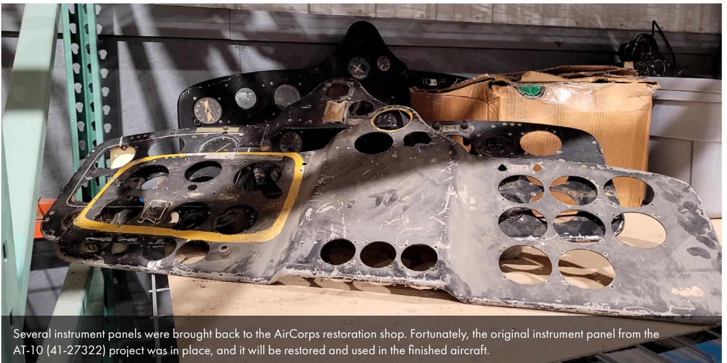
Several instrument panels were brought back to the AirCorps restoration shop. Fortunately, the original instrument panel from the AT-10 (41-27322) project was in place, and it will be restored and used in the finished aircraft.
