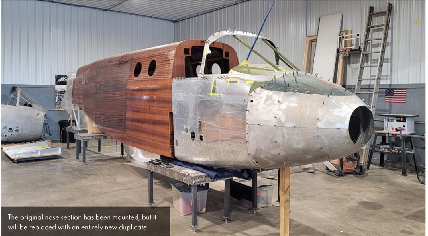
The original nose section has been mounted, but it will be replaced with an entirely new duplicate.
