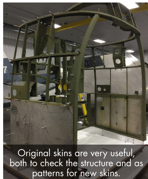
The basic cabin area structure on an AT-10 is some of the limited metal structure. Here the framework has been painted and reassembled.
