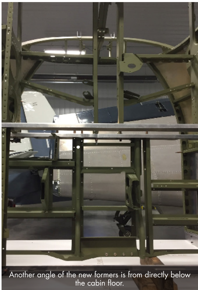
The basic cabin area structure on an AT-10 is some of the limited metal structure. Here the framework has been painted and reassembled.
