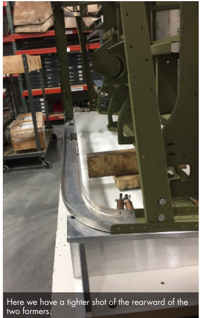
With the aluminum clamped between two MDF forms, Guy gradually shapes the fuselage former with a plastic hammer.
