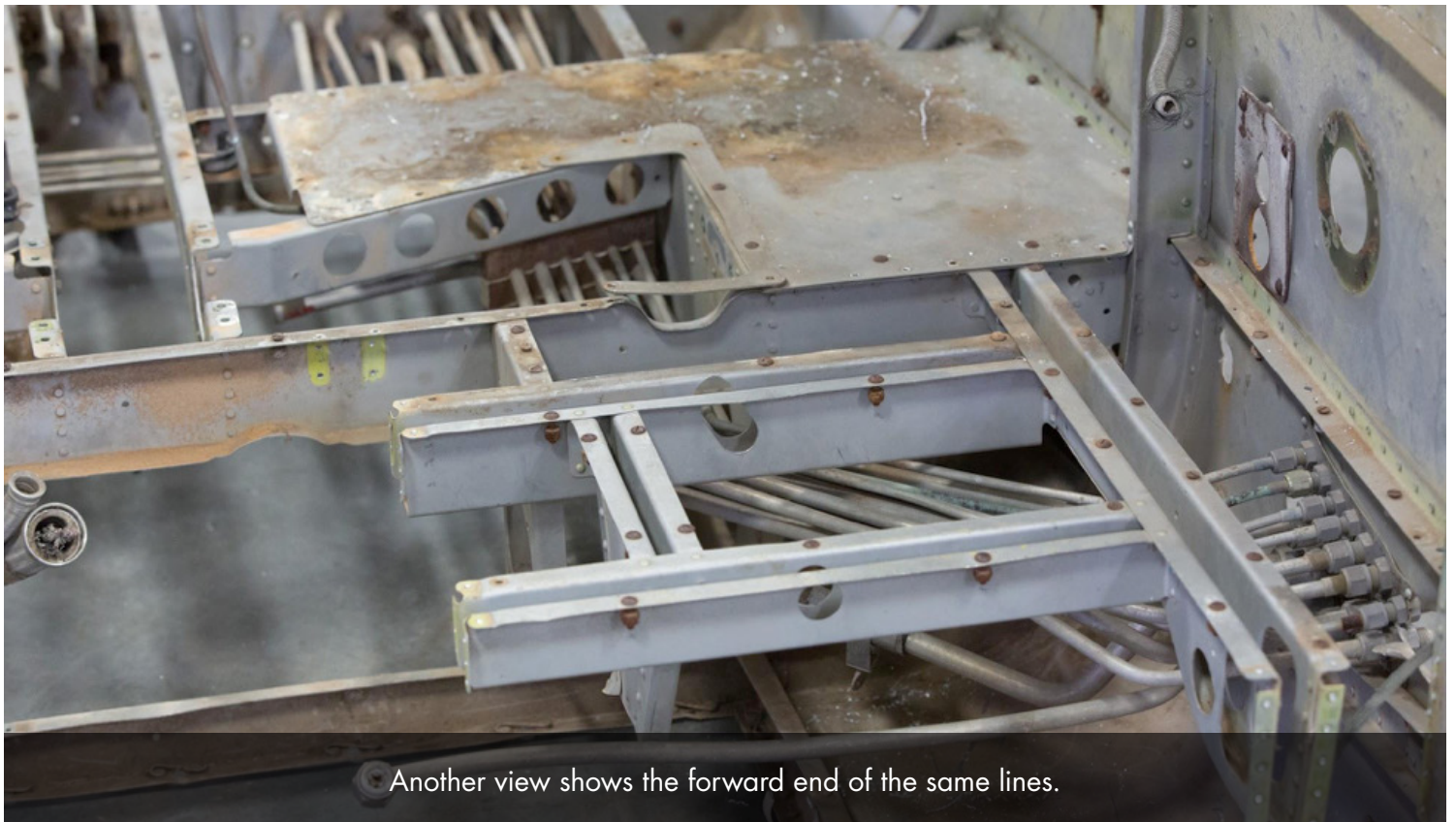
This tight view shows some of the hydraulic lines that run under the cockpit floor.
