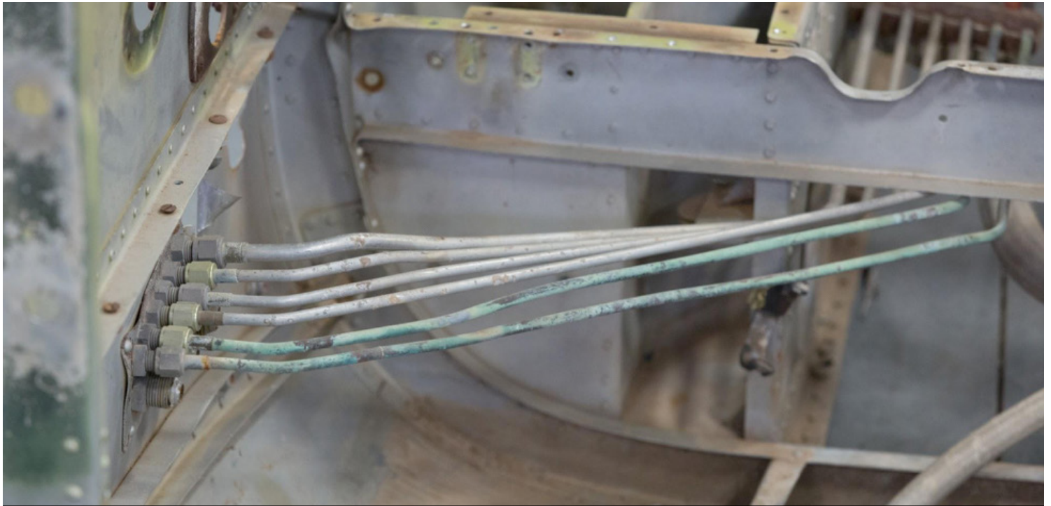
This tight view shows some of the hydraulic lines that run under the cockpit floor.
