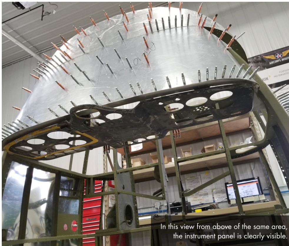
Here, the skin for the glare shield is being fitted to the frame and instrument panel. The line marked in black shows where the edge of the windshield frame will be located.
