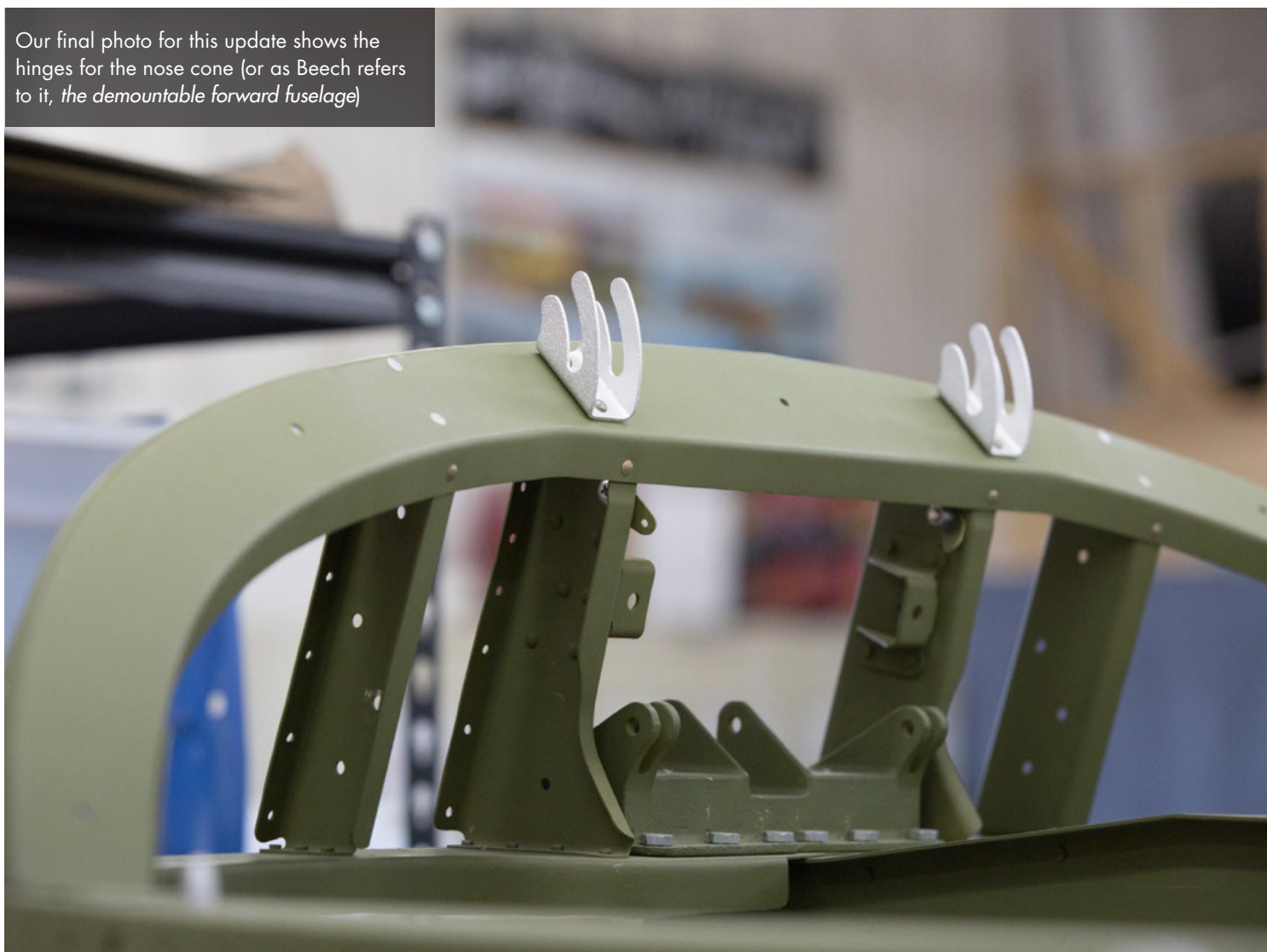
The forward most skin section of the glare shields also shows the lines marking the future location of the windshield frame edges.
