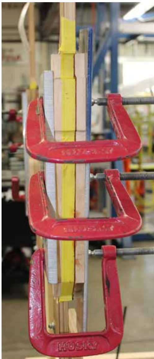
Many clamps are necessary to provide even gluing pressure.
