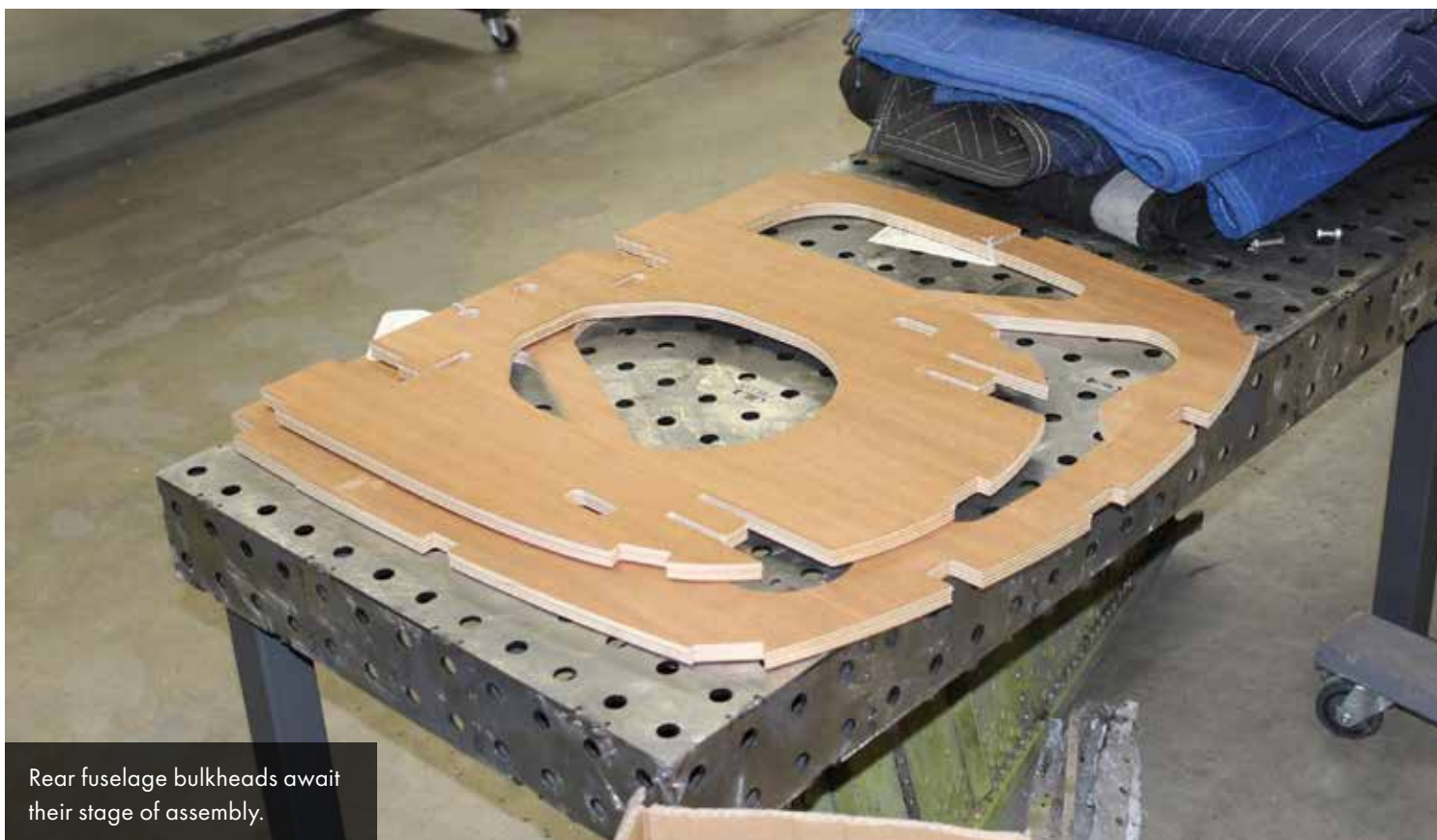
Precision milled parts are necessary to build a precise airframe.
