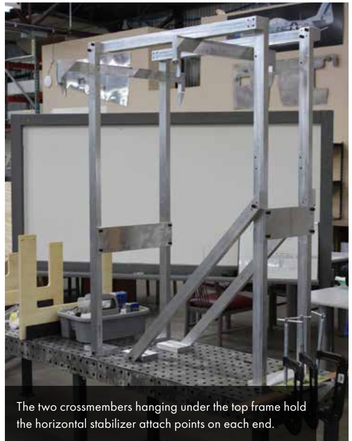
The last three stations on the fixture are encompassed in this heavy aluminum frame because they are positioned high above the fixture table and include mounting points for the horizontal stabilizer, three frames, and the tail wheel.
