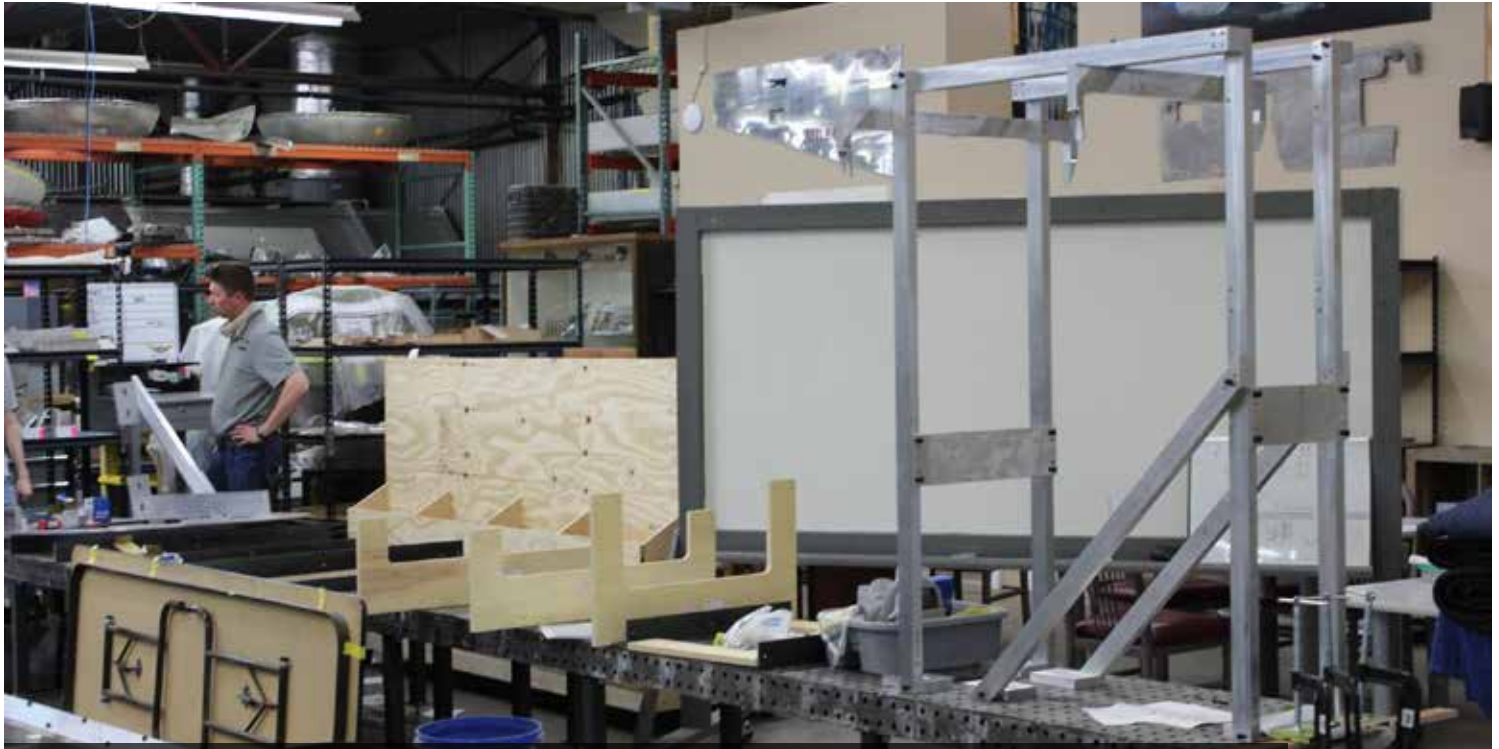
The last three stations on the fixture are encompassed in this heavy aluminum frame because they are positioned high above the fixture table and include mounting points for the horizontal stabilizer, three frames, and the tail wheel.
