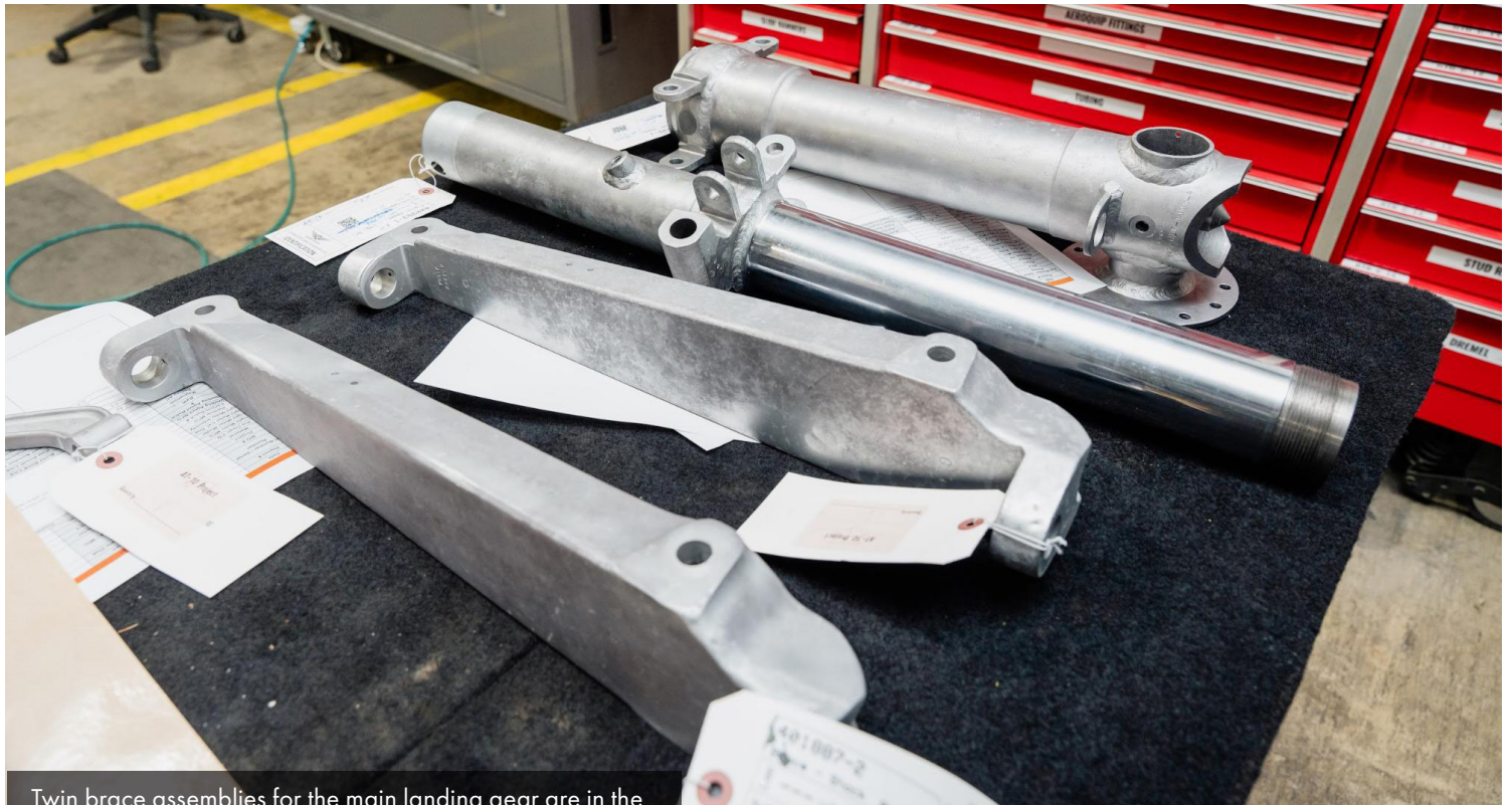
Twin brace assemblies for the main landing gear are in the foreground, with struts in the background.
