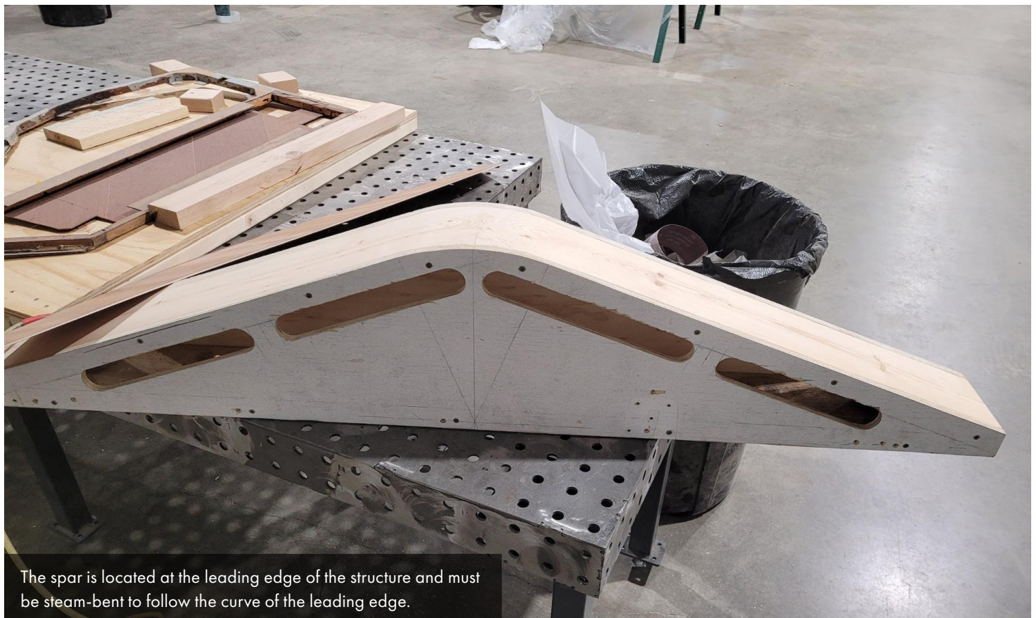
These are spruce blanks for fabricating the main horizontal spar.
