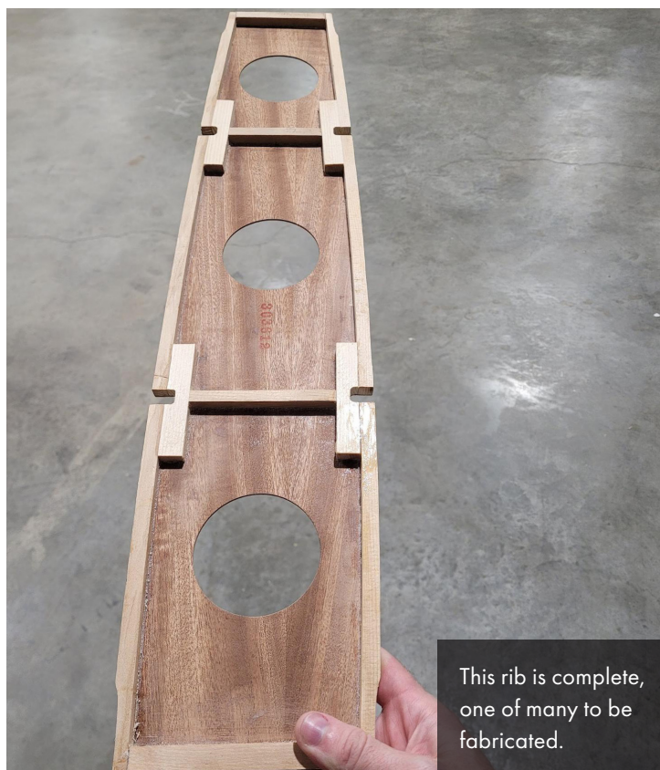
Vertical stiffeners are glued and clamped to set.
