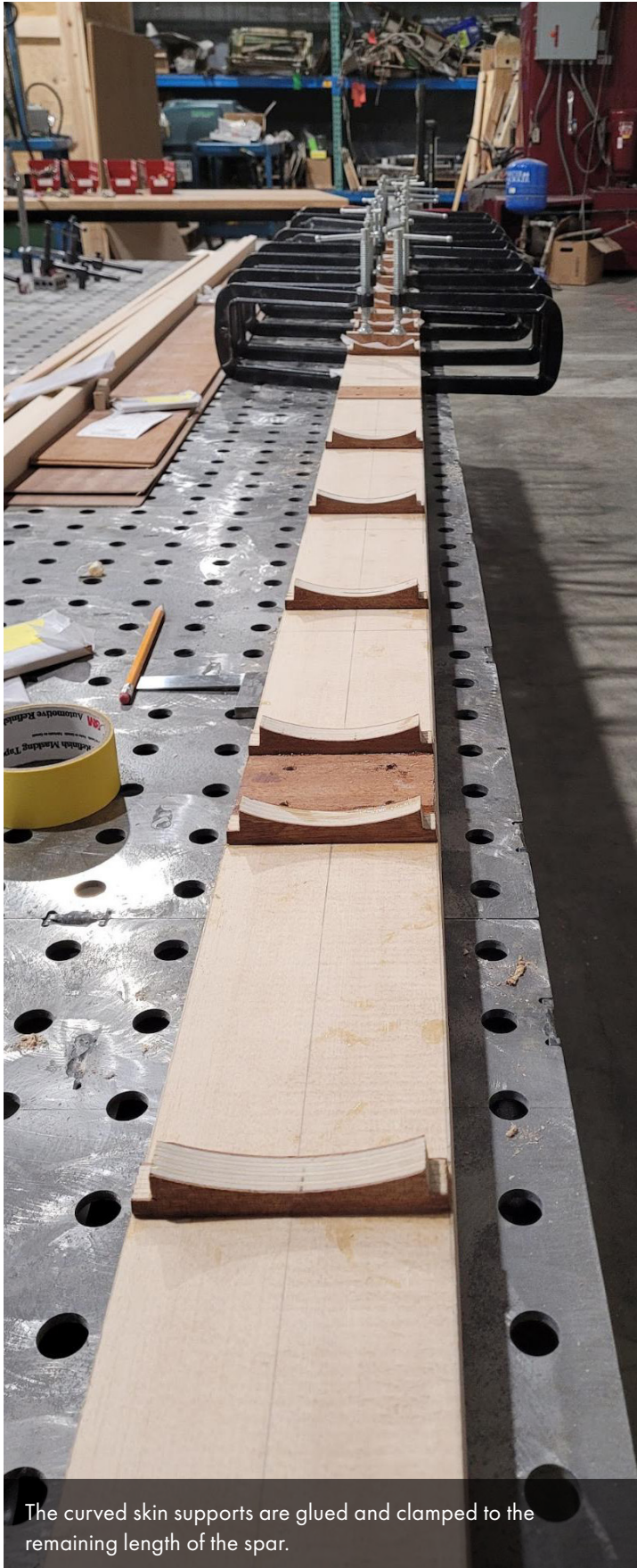
This view shows all the skin support pieces permanently installed in their correct locations along the entire spar.
