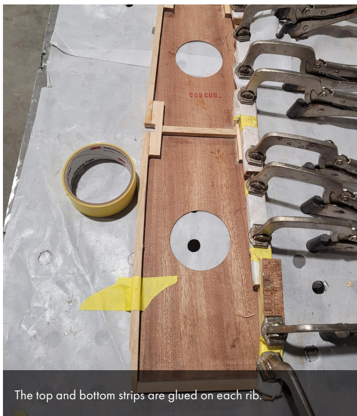
The next task Aaron undertook was to make ribs for the horizontal. The ribs are thin plywood stiffened by spruce strips.
