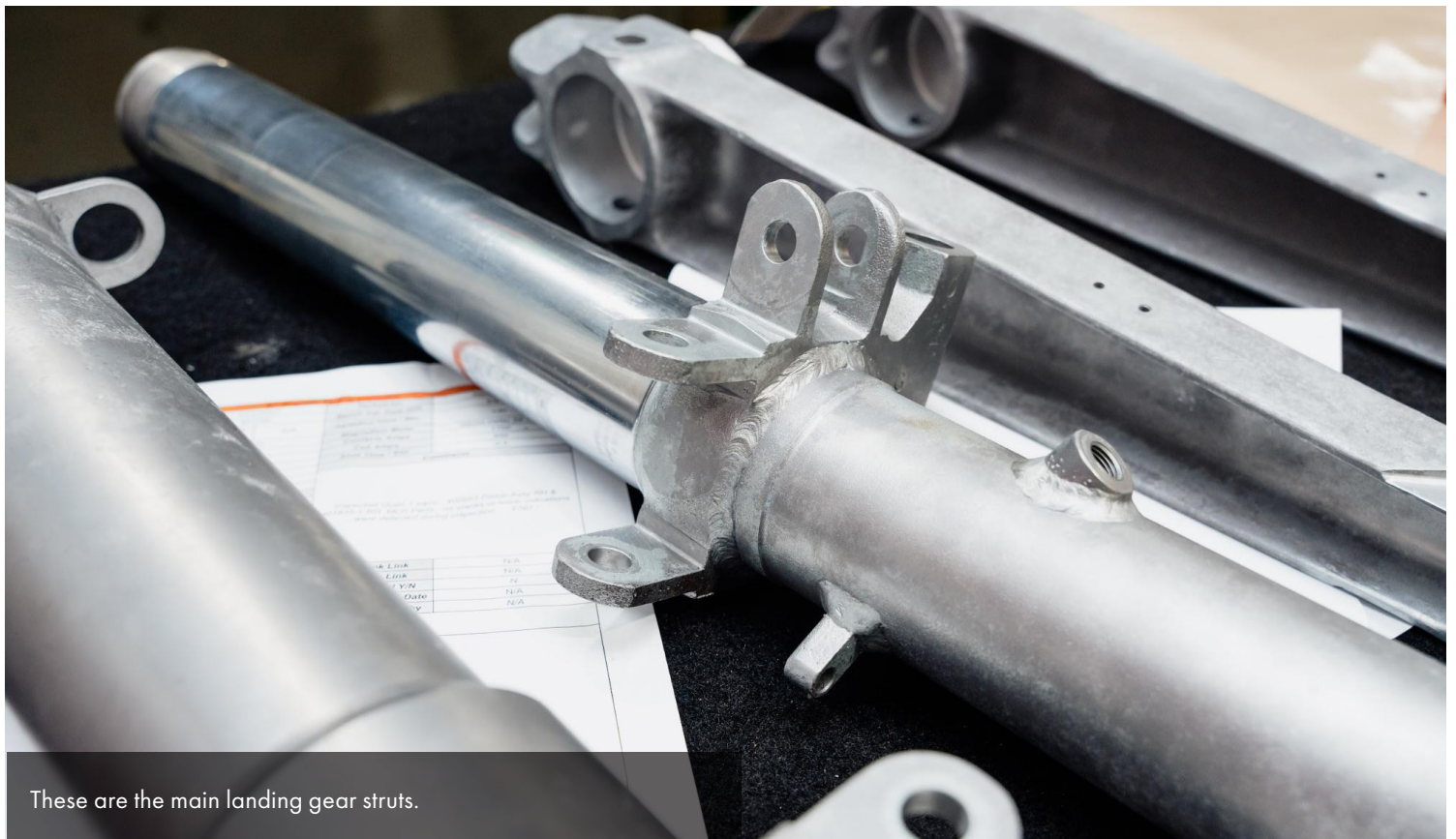
Twin brace assemblies for the main landing gear are in the foreground, with struts in the background.
