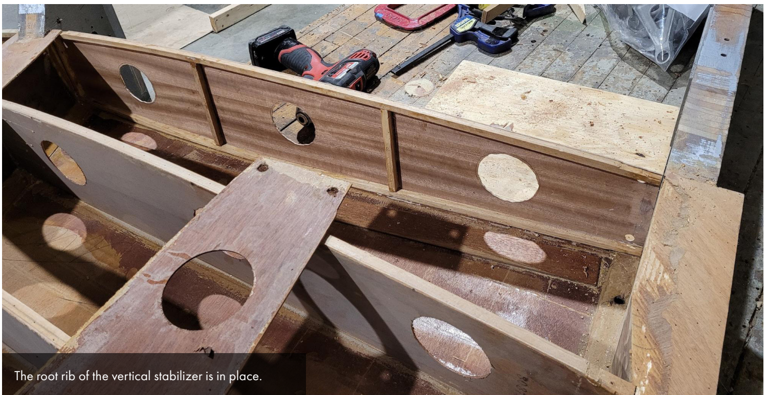
In this photo, the spruce cap strips and upright strips were glued and clamped to the plywood part of the root rib.
