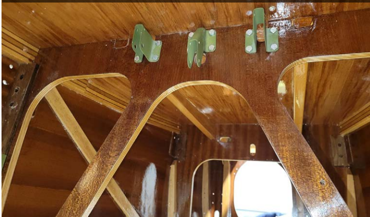
These brackets will hold pulleys for the control system. The brackets on the left and right are for rudder control cable pulleys. The center bracket holds the elevator control cable pulley.
