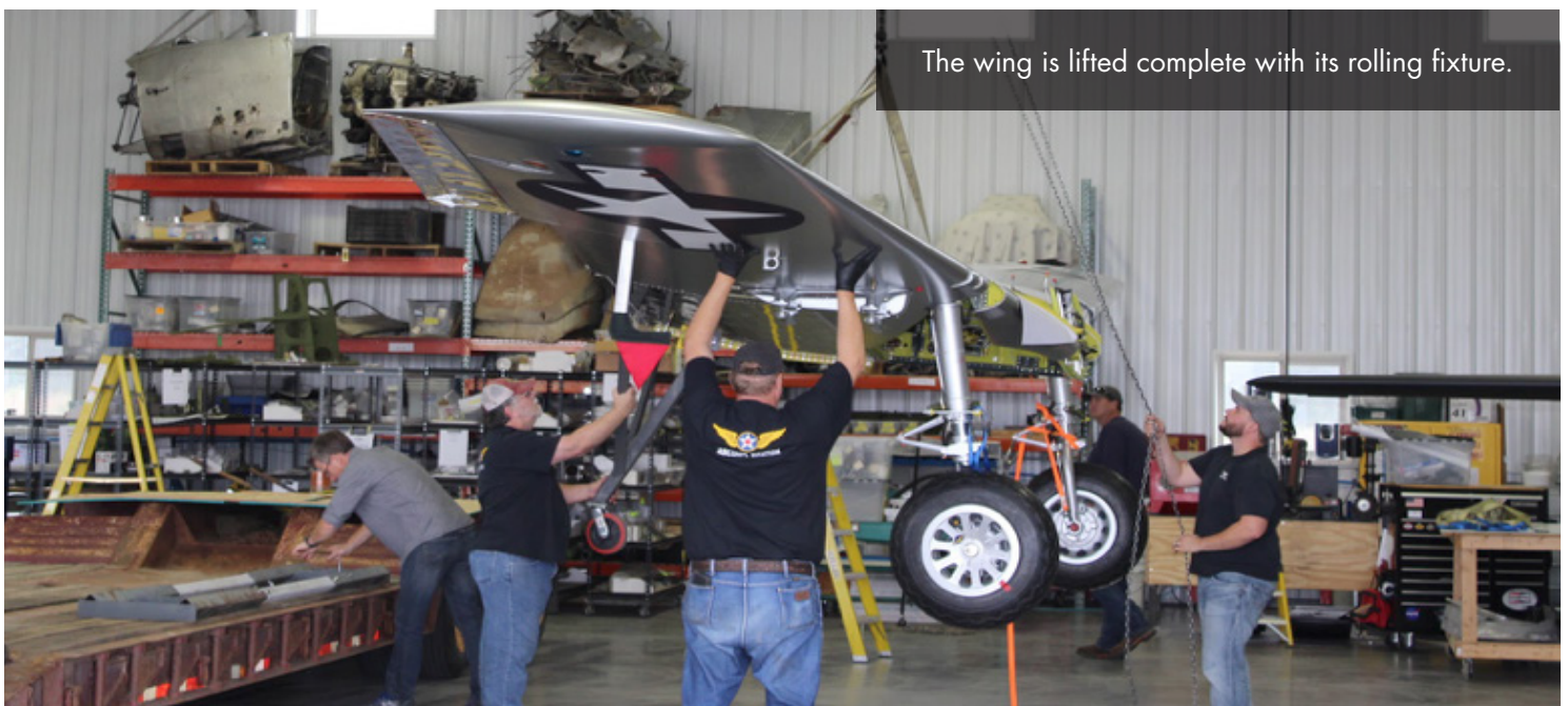
The center of the wing is situated under the lifting beam and hoist.
