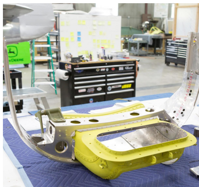
This induction elbow connects to the carburetor.
