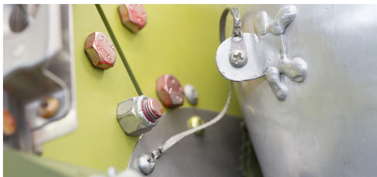
The ground strap on the oil tank is small but essential.
