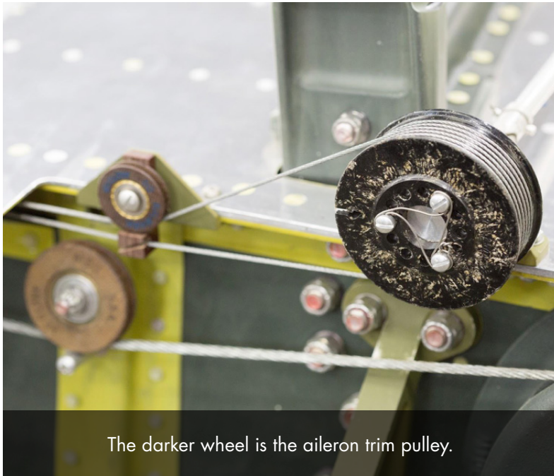
The larger cables are for the left side aileron and the small ones are trim tab cables.
