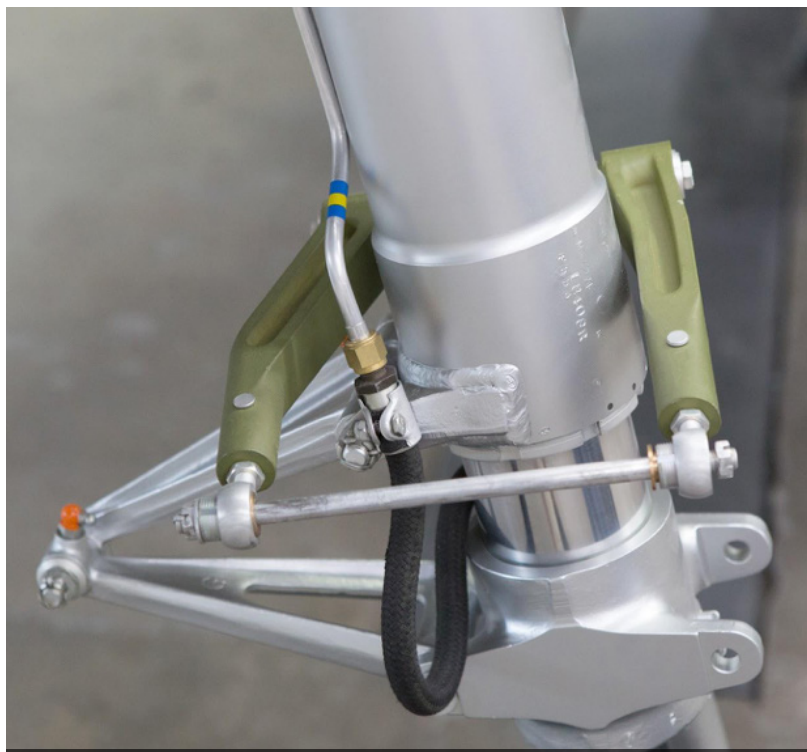
The Bendix landing gear shock strut is painted silver and the green linkage is used to connect the outer gear doors to the shock strut.
