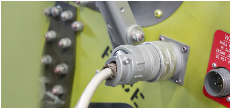
The connector at the terminus of the wire is the generator disconnect cannon plug.
