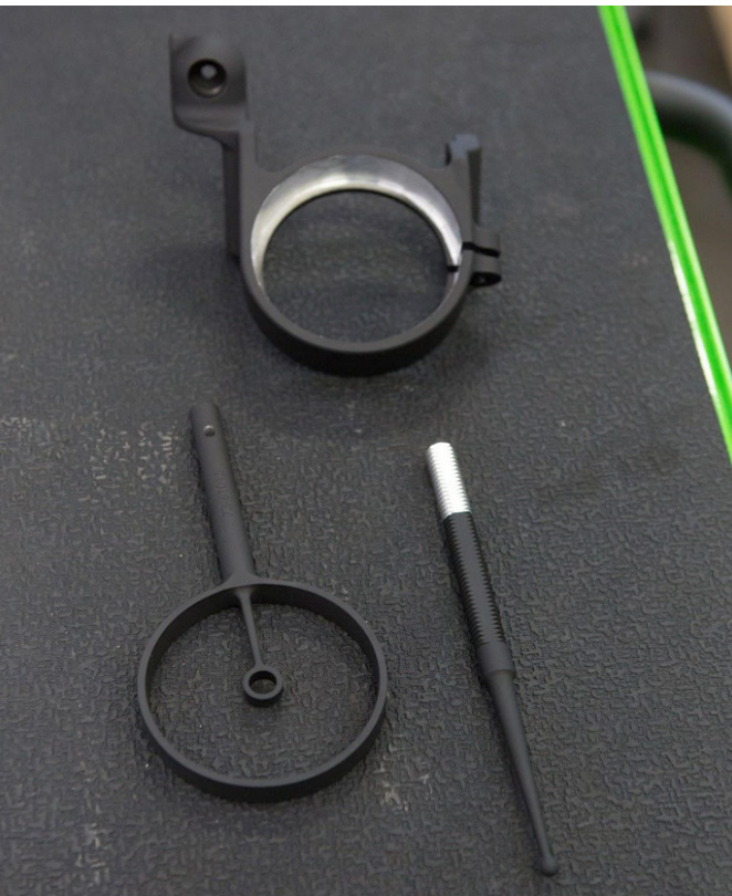
Auxiliary gun sights; the bead sight is mounted to the firewall and sticks up from the top cowl. If the bulb burned out in the optical sight, or other damage occurred, the pilot still had a way to aim his four 50 caliber guns.
