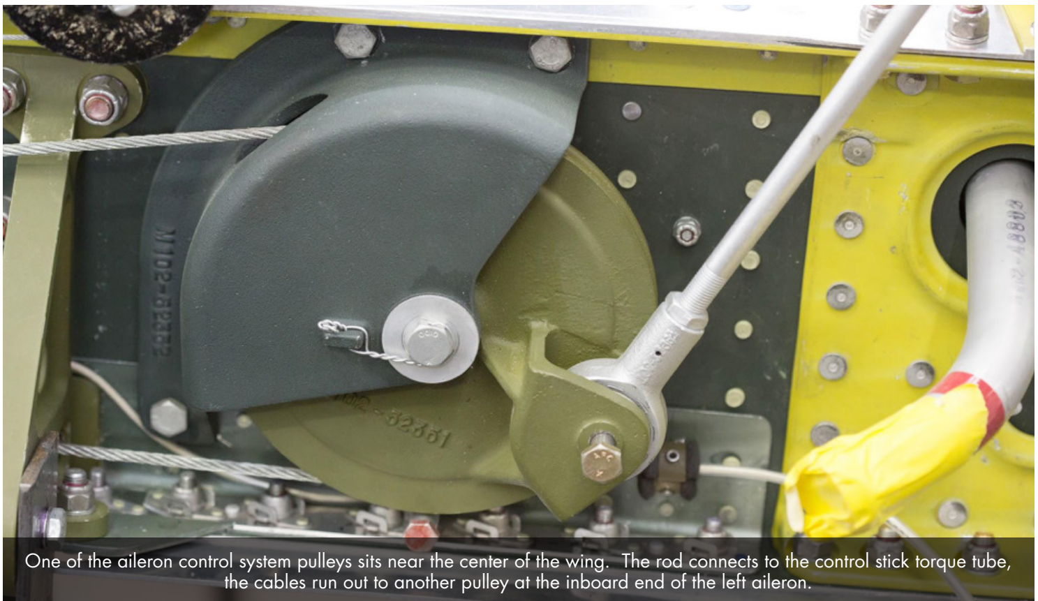
The larger cables are for the left side aileron and the small ones are trim tab cables.
