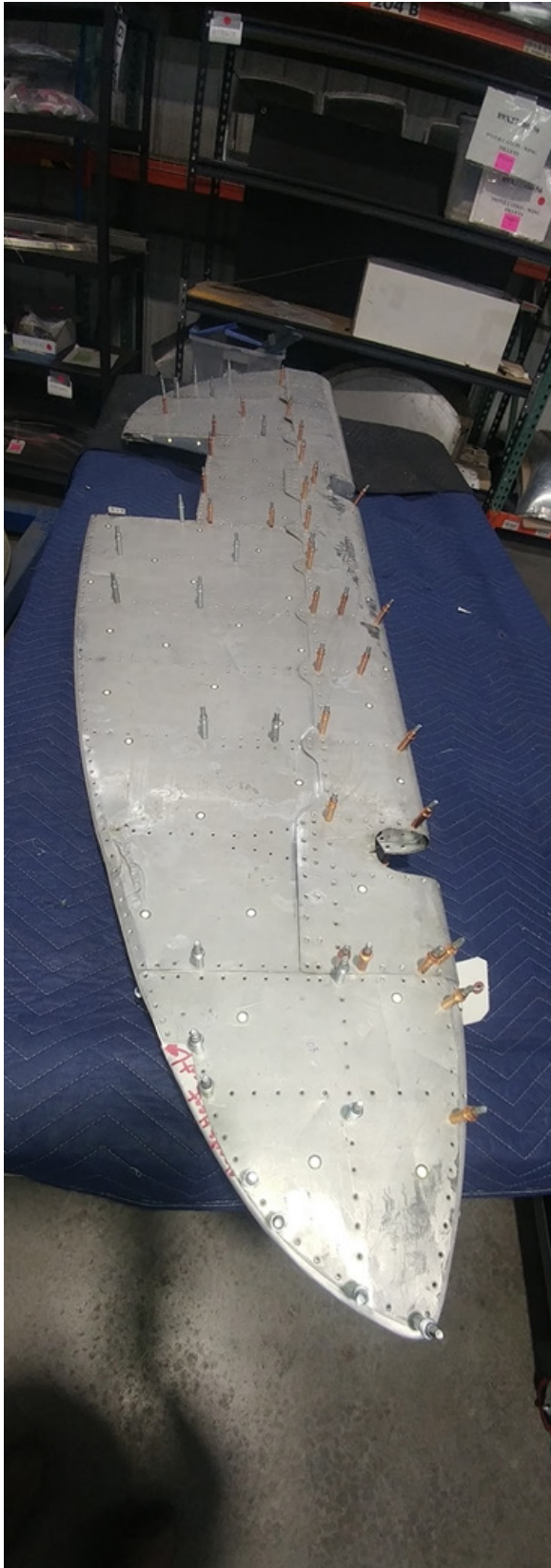
This particular elevator has been temporarily reassembled so that it can be 3D scanned.
