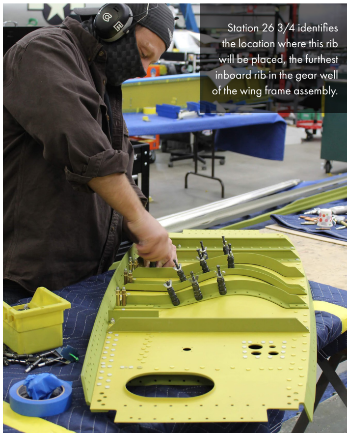
Brad works on 89C22121-54 rib assembly, station 26 \frac{3}{4} . It joins Spar #1 to Spar #2
