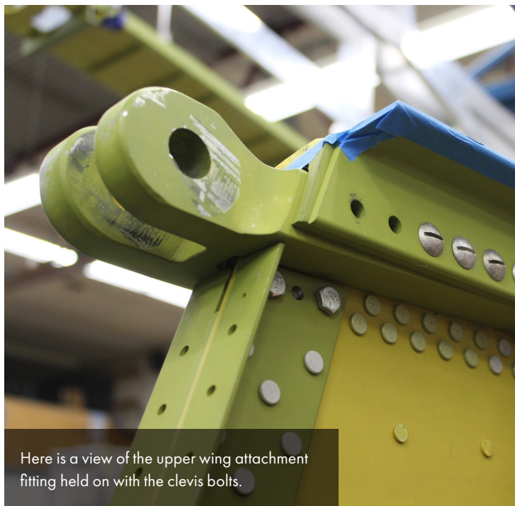
The darker green components are vertical stiffeners riveted to the main spar.
