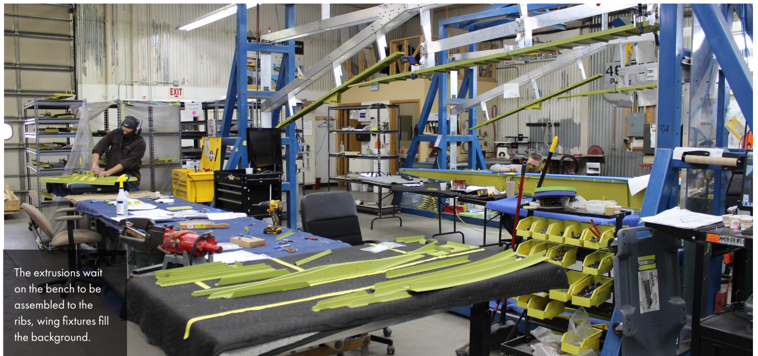
These extrusions have been painted and are ready for the large rib assemblies from the gun bay to the gear well area - Stations 64 to 132.
