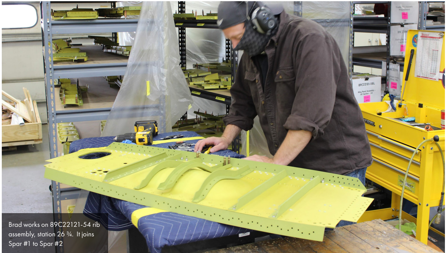
Station 26 \frac{3}{4} identifies the location where this rib will be placed, the furthest inboard rib in the gear well of the wing frame assembly.
