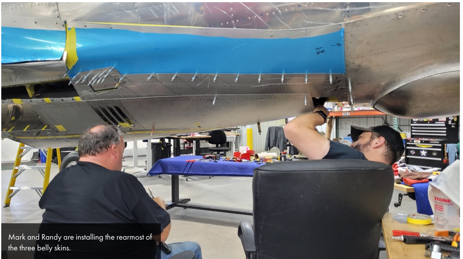
Finally, here is the rearmost of the three belly skin sections.
