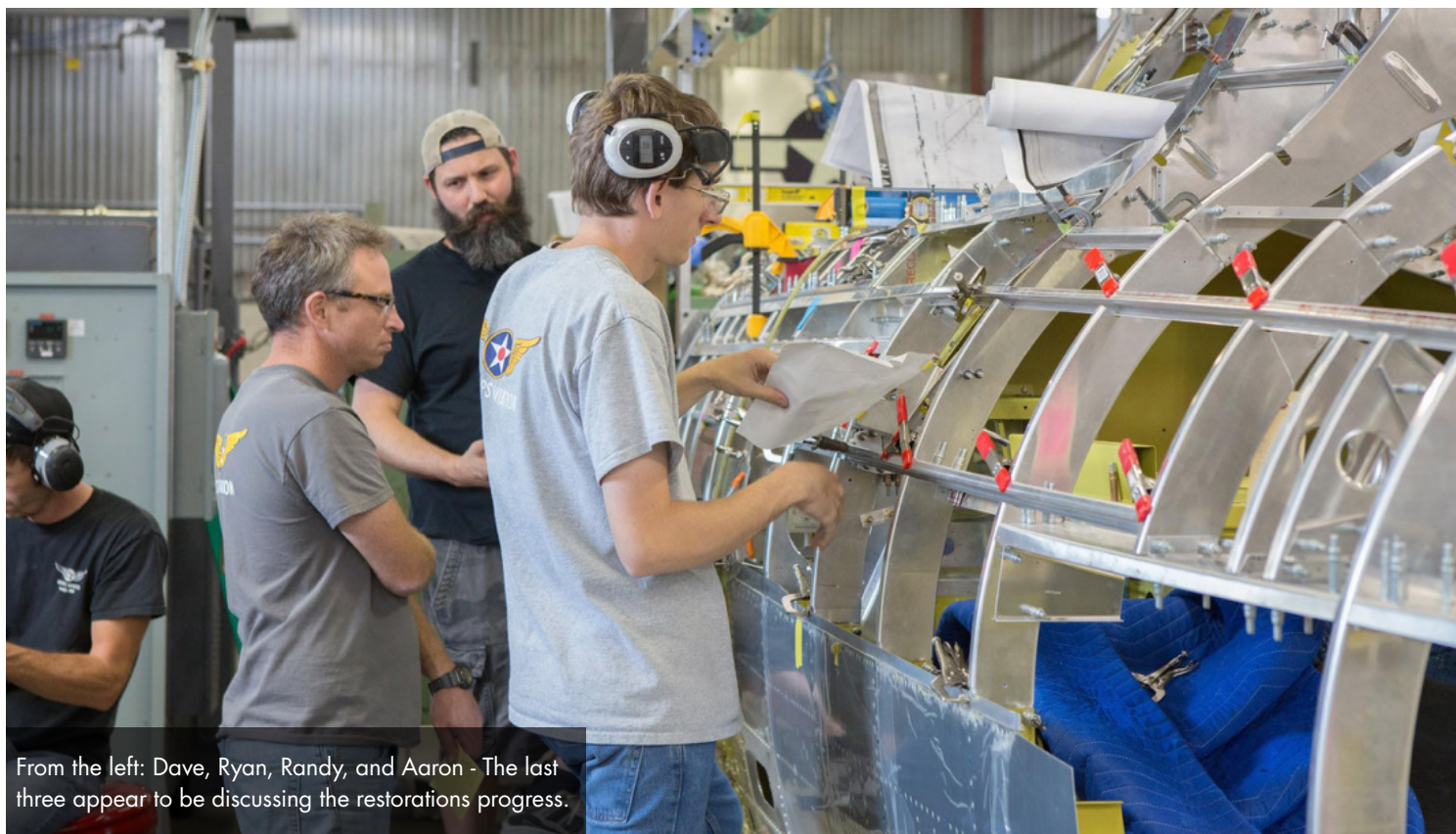
As assembly gets more detailed, the guys insert engineering drawings into handy spaces in the structure for quick reference.
