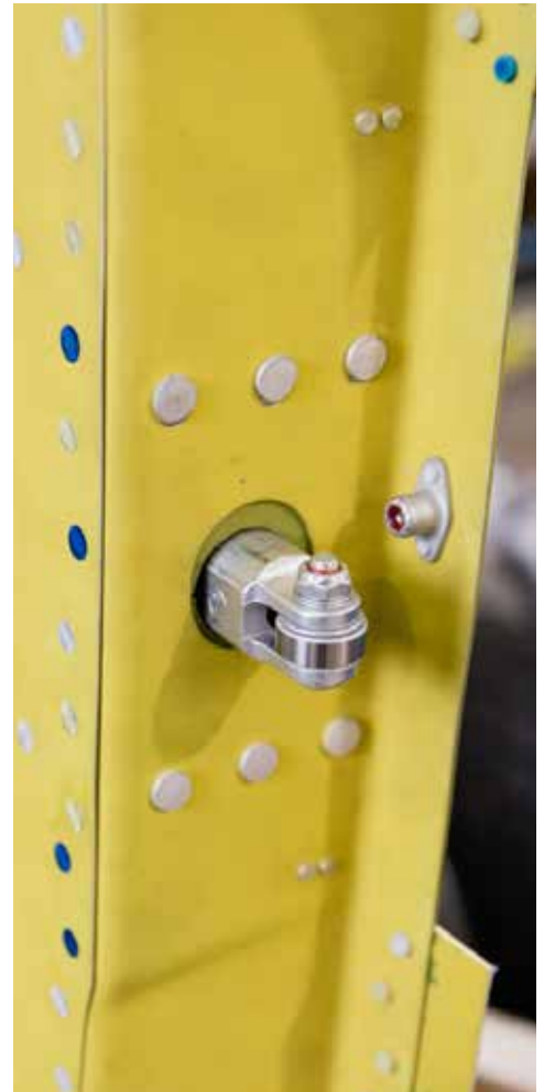
The door lock mechanism protrudes from the wheel fork fairing.
