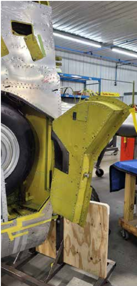
The inner skin for the wheel fork fairing has been installed.
