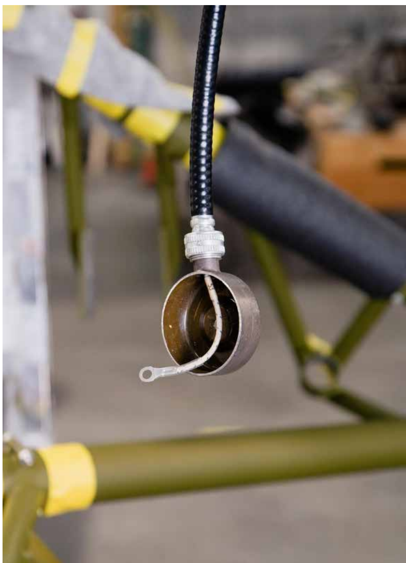
This electrical harness and cap connect to the oil dilution solenoid. Oil was slightly diluted with gasoline from the fuel tanks for cold weather starts.
