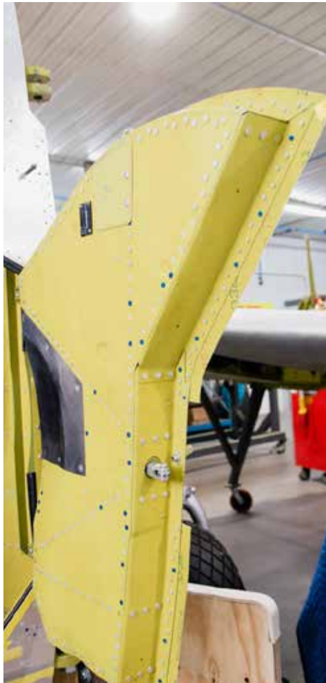
Here is a closer look at the details of the wheel fork fairing.
