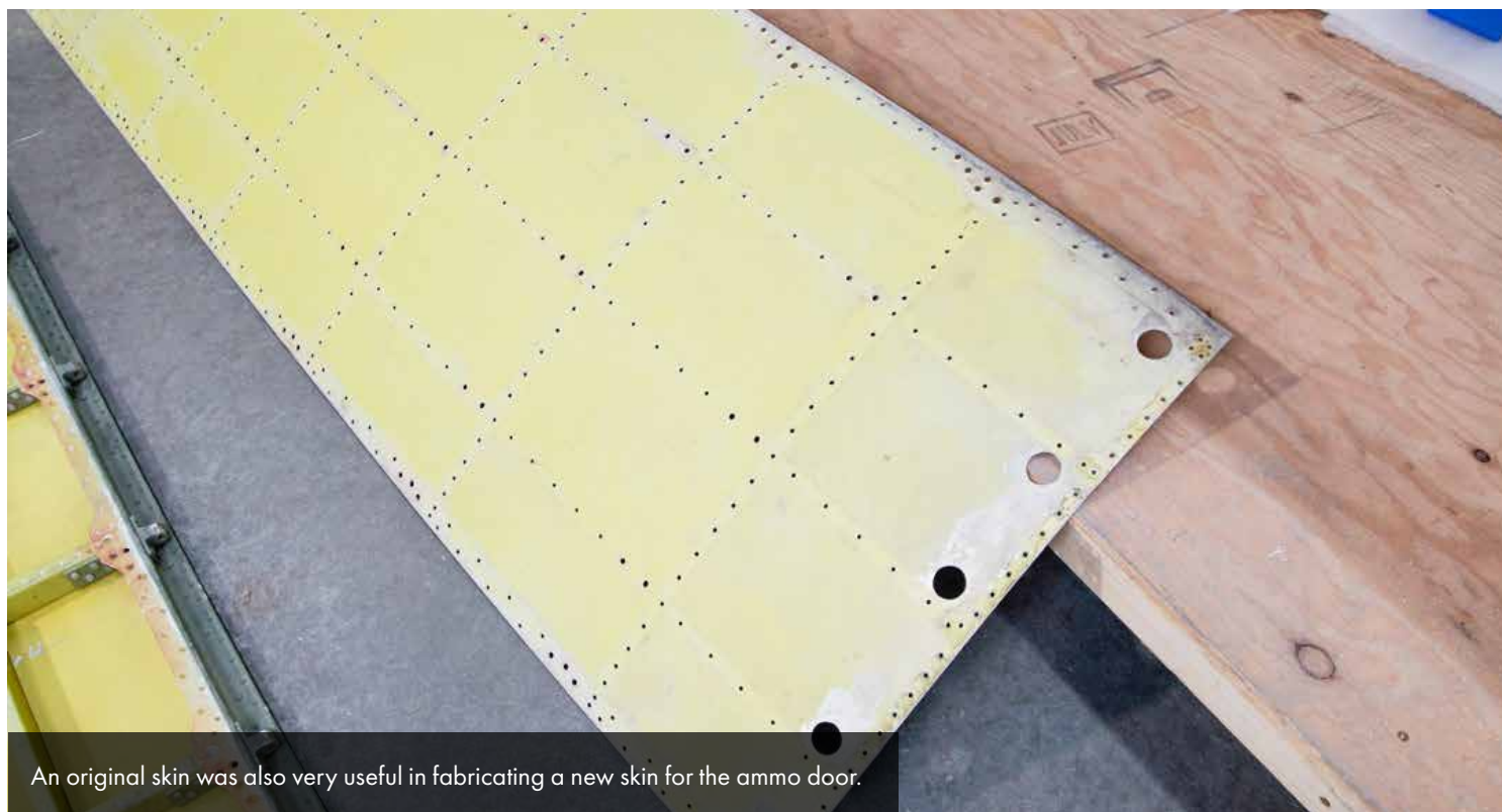
An original ammo bay door was used as a template for the new assembly.
