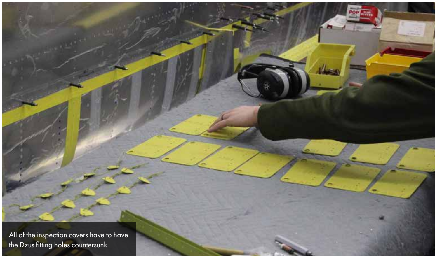
Corey works on inspection hole covers that will cover the openings visible in front of the flap and aileron positions near the top of this photo.
