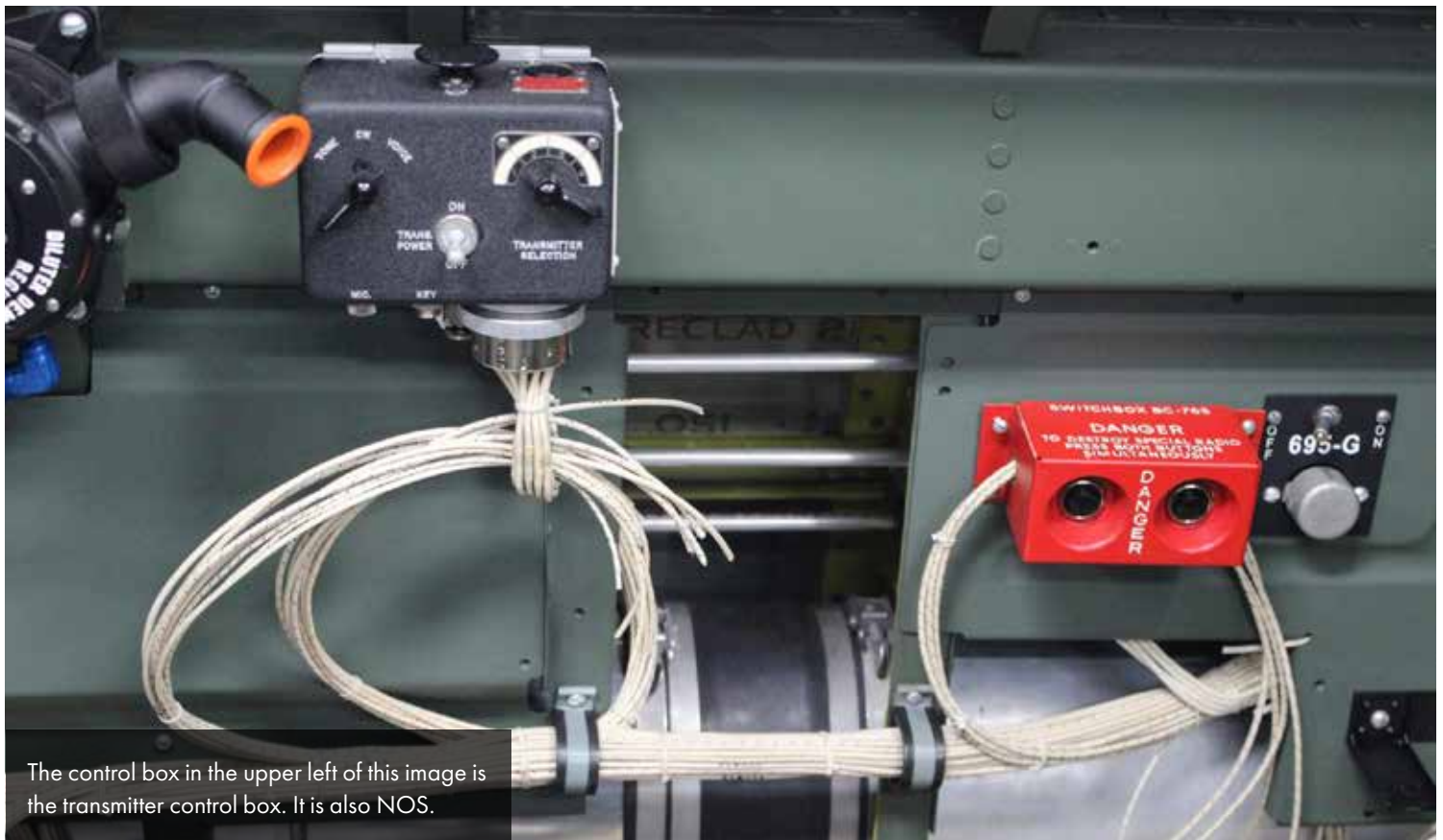
This close up shows some of the detail on the IFF manual self destruct control. This part is a NOS (new old stock) part that was located in its original box, untouched since it was manufactured during the war.
