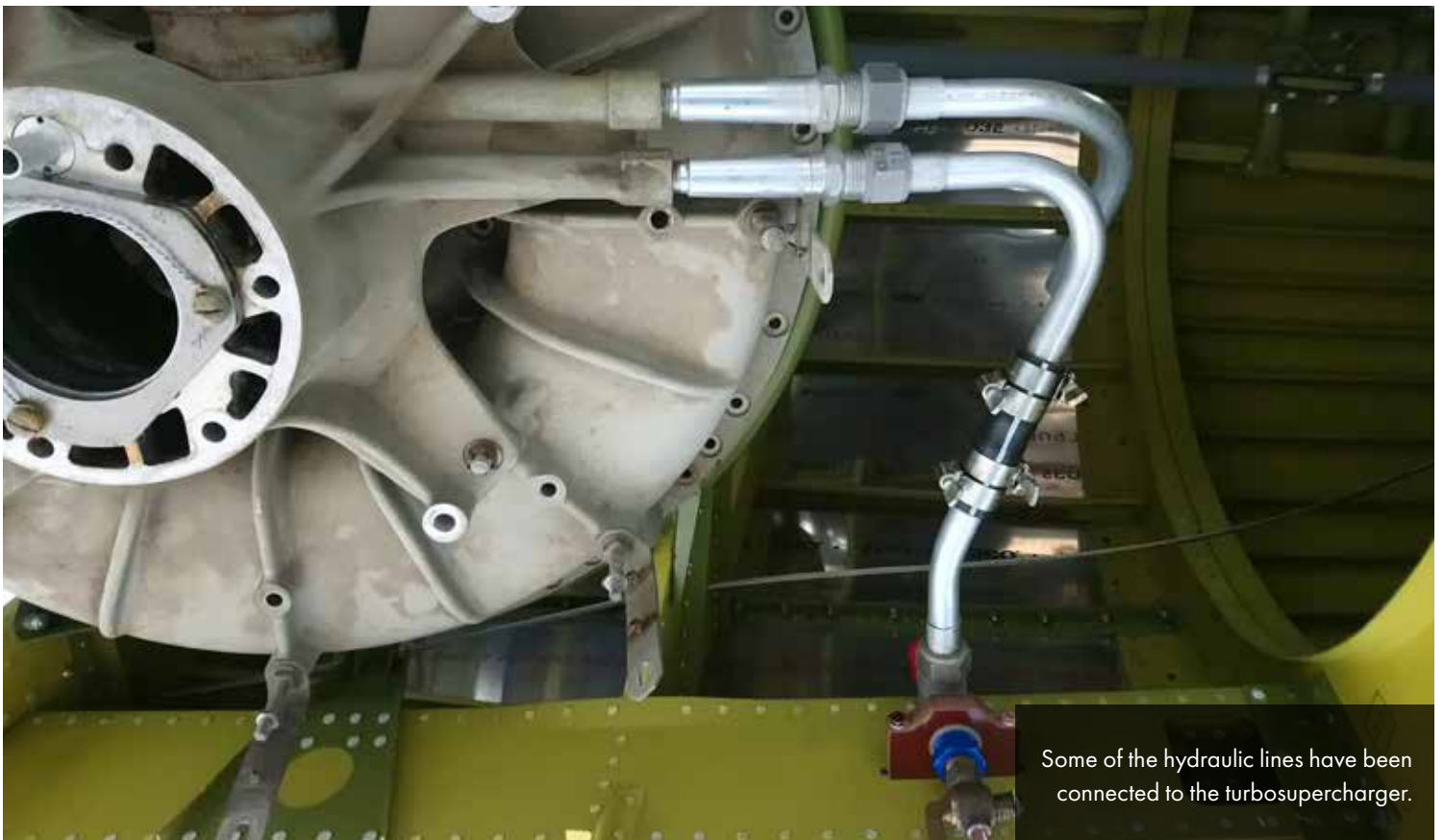
The turbosupercharger and associated ducting is the reason for the deep fuselage on the P-47.
