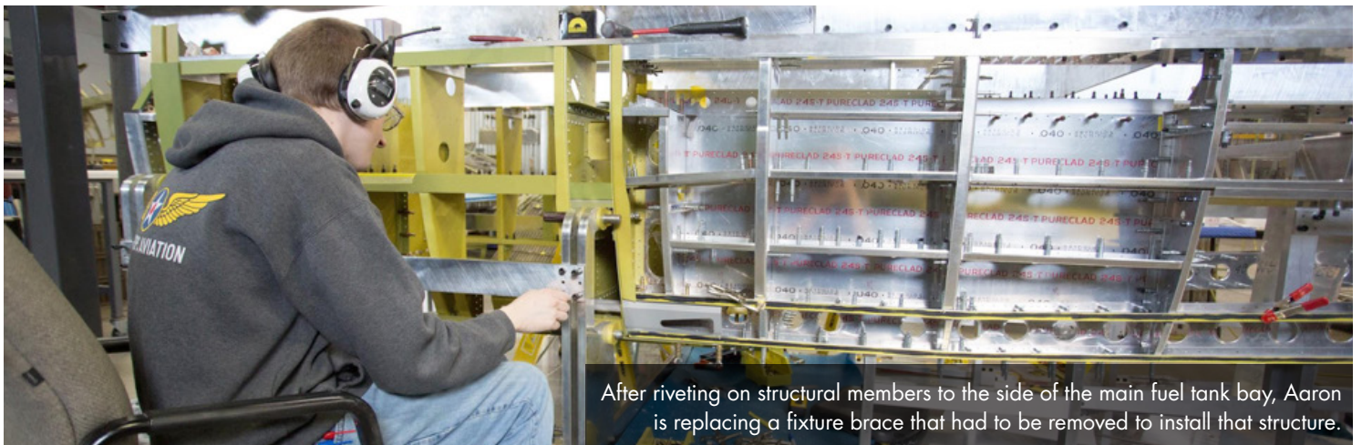
The main fuel tank space's relationship to the rest of the fuselage structure is clear in this image.
