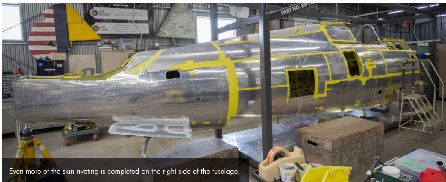
This quartering angle shows us how much of the left side fuselage skin is riveted on permanently.
