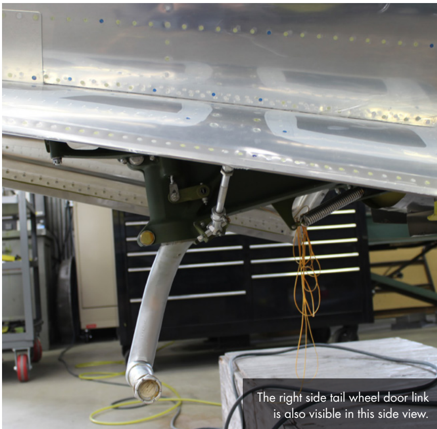
The darker green casting is called the tail wheel drag brace and pivots up as the tail wheel is retracted.
