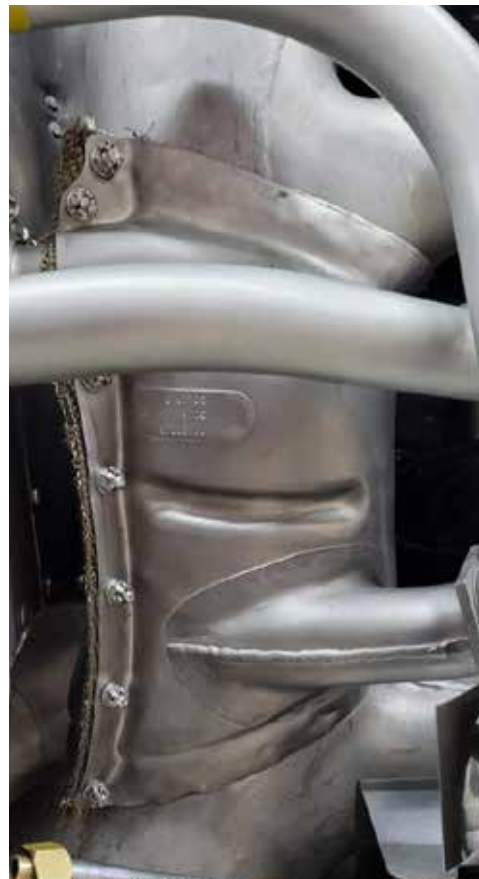
This is the heater muff assembly that mounts to the exhaust manifold on the right side. It takes heat from the manifold and passes it on to the cockpit heater and windshield defroster.
