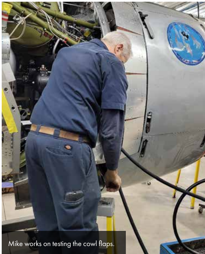
The hydraulic "mule" (in the bottom of the photo slightly left of center) is hydraulically connected to operationally test the cowl flaps.
