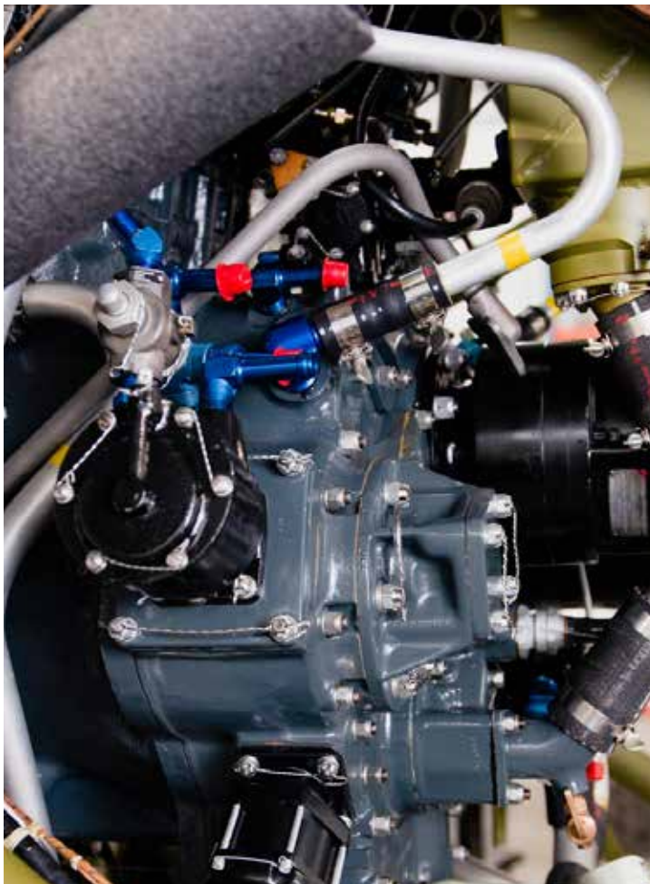
In this view of the gray accessory case, the vacuum pump is visible. It is a black assembly with safety wired cover screws.
