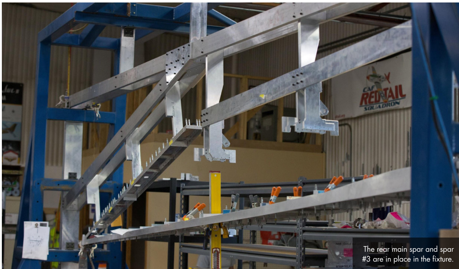
The part with the holes is the reinforcing plate for wing Rib #64.
