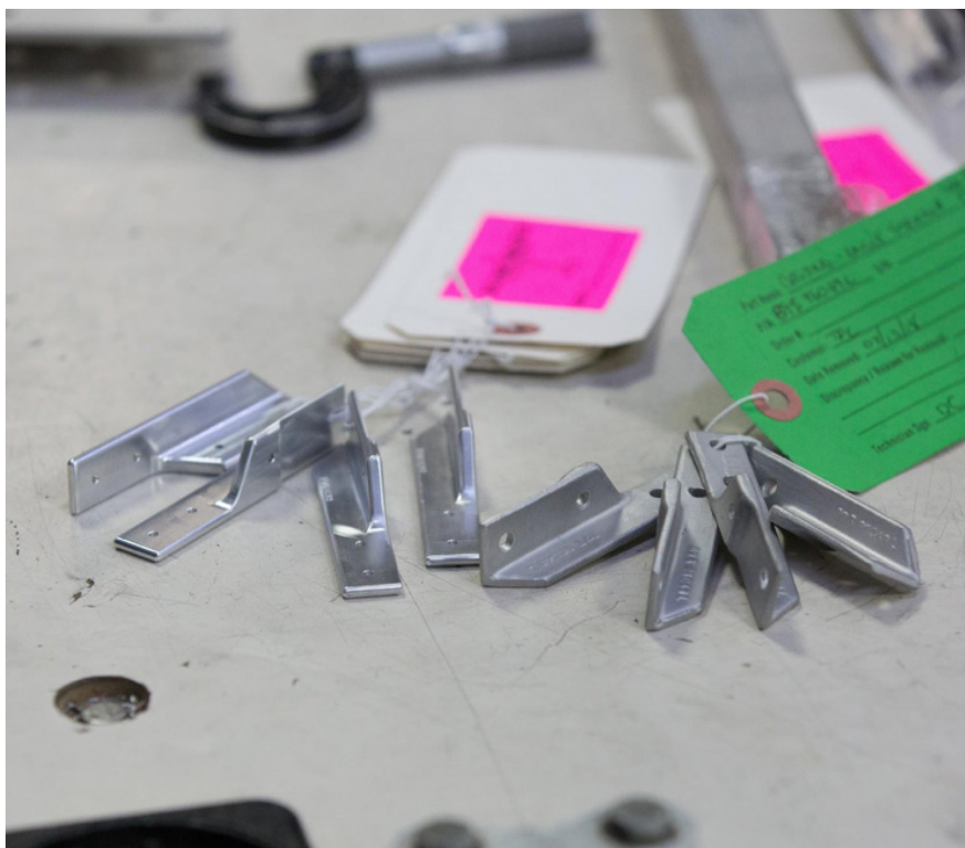
The engineering drawings label these as CSTG (casting) clip 89S96049R, stringer station 2.02
