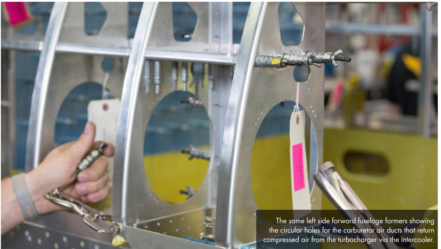
One of the guys works on an upper fuselage former located just behind the firewall.
