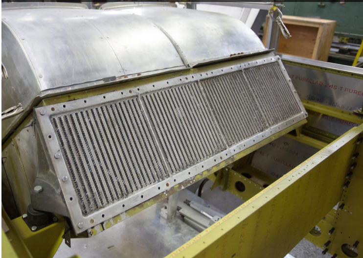
The intercooler takes in hot, compressed air from the turbocharger, cools it, and sends it back forward to the carburetor from this side.
