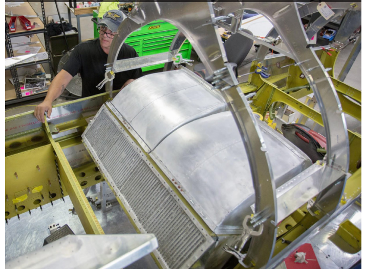
A longer shot shows Robb next to the intercooler cool air exit and we can see its relationship to the fuselage structure.
