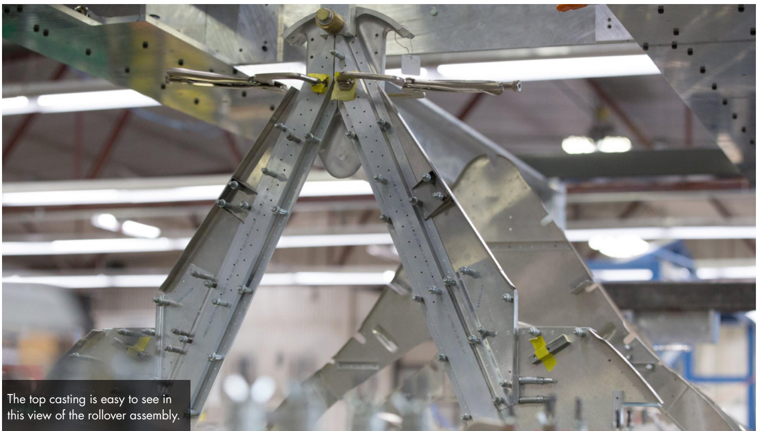
A view from the rear of the same assembly shows the top piece being fitted.
