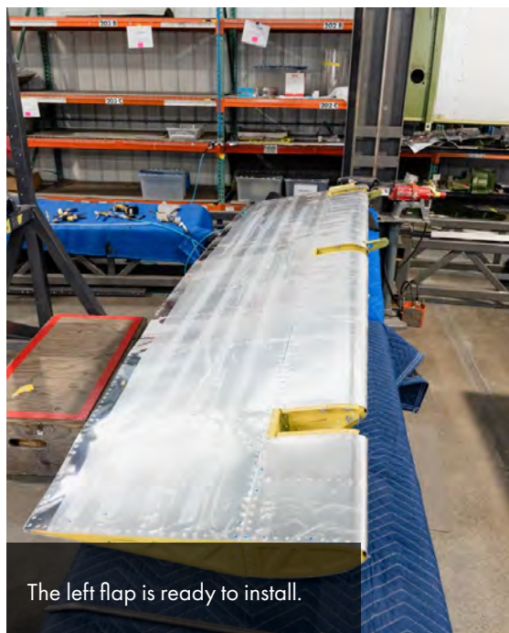
Randy and Cory prepare to remove the finished left flap from its fixture.
