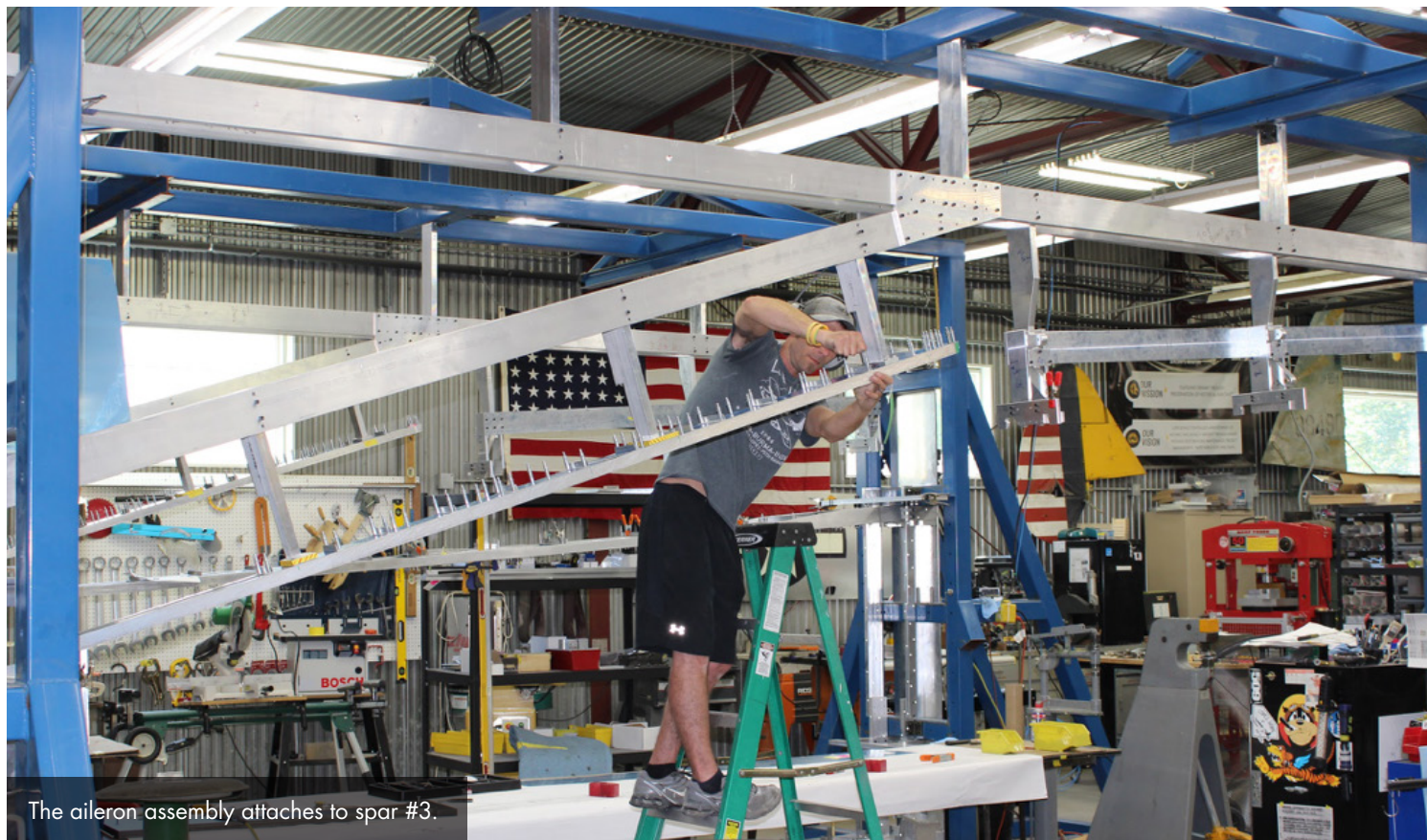
Dave inserts a cleco in the outboard #3 spar on the right wing. In the background the main spar and outboard spar #3 for the left wing are visible.
