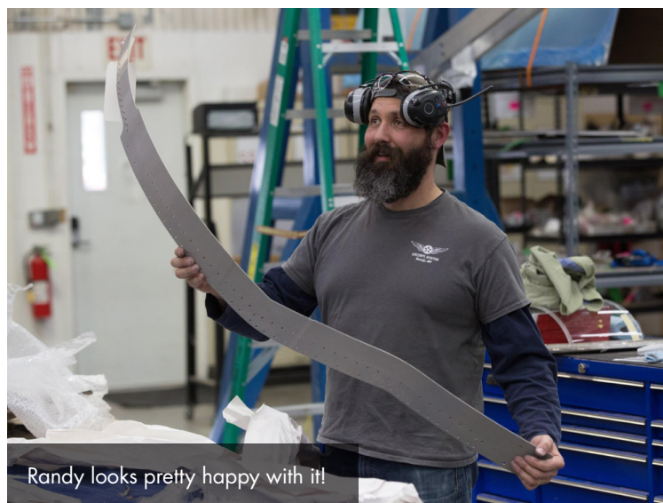
This extrusion is the front edge of the firewall extension and has a series of complicated bends that Randy made before sending it out.
