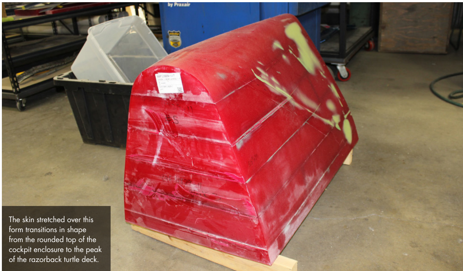
This large REN plastic form was machined to stretch form the rear window cover, part of the cockpit enclosure.
