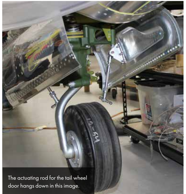
The tail wheel doors are installed, but have yet to be connected to their actuating system.
