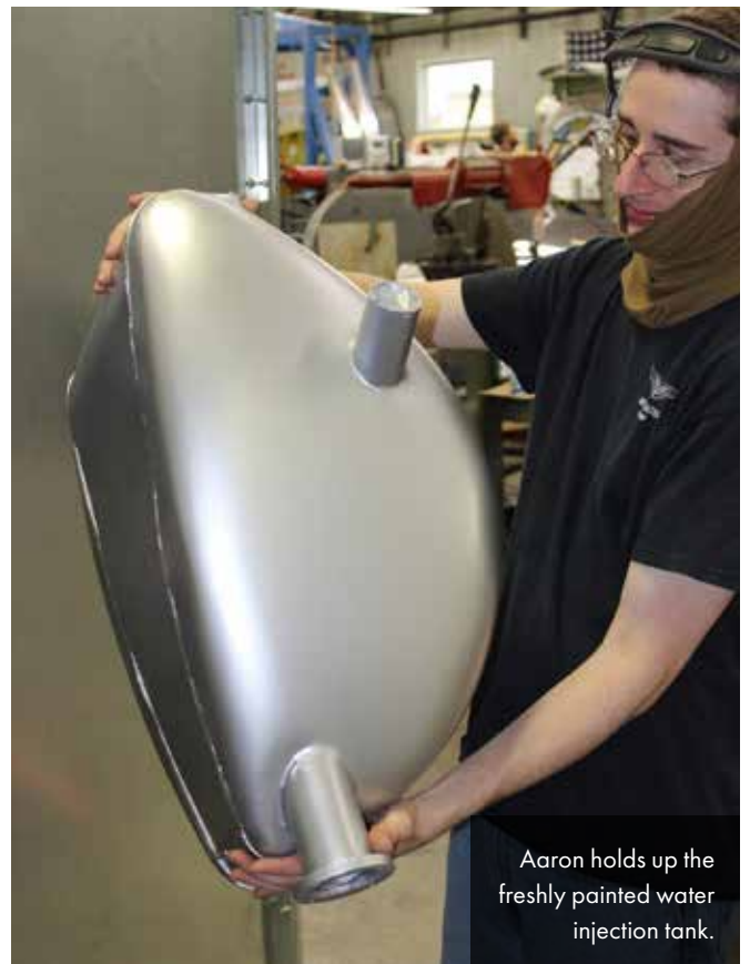
The water injection tank has been painted the correct silver color.
