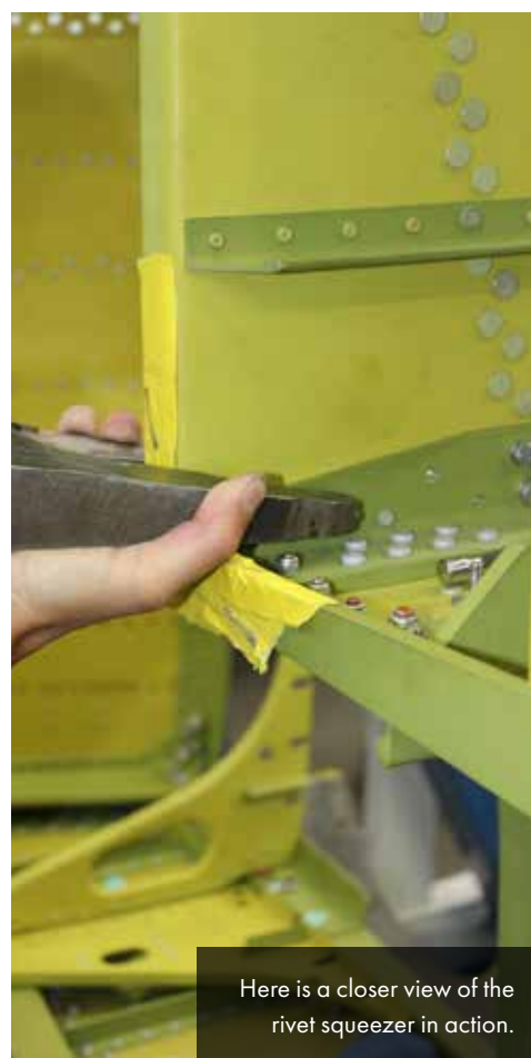
Cory rivets the auxiliary landing gear spar, which supports and braces the landing gear bearing box.
