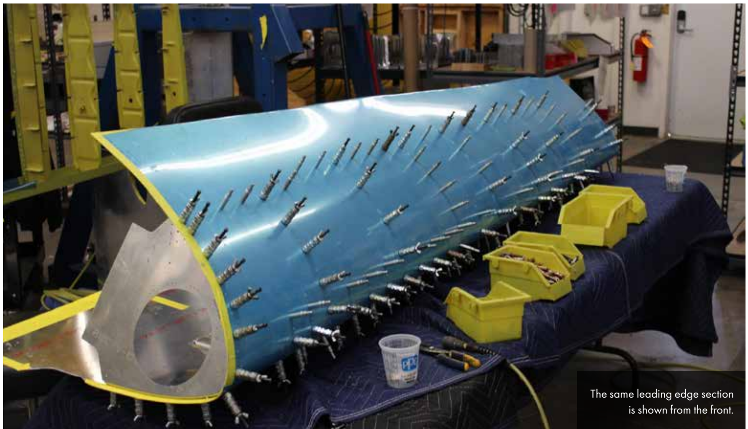
The inner leading edge, seen here from the rear, is much thicker than the outer leading edge section.
