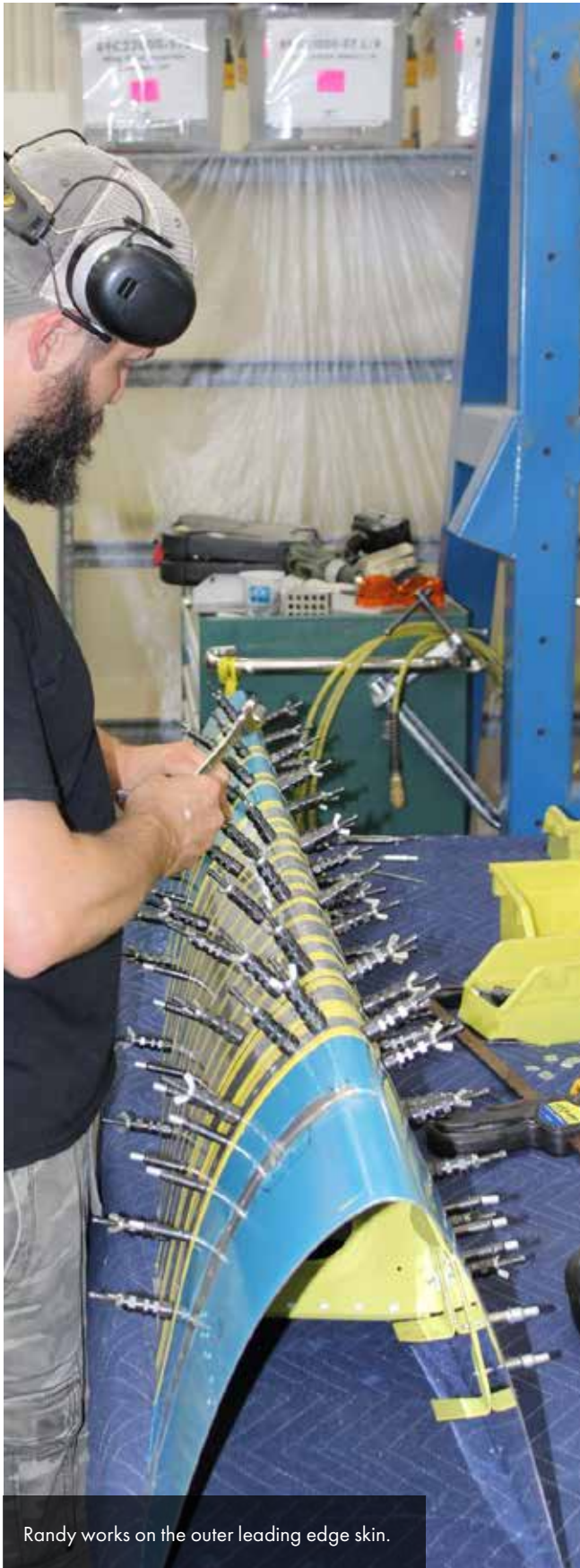
The painted inner structure is visible in this view of the outer leading edge section.
