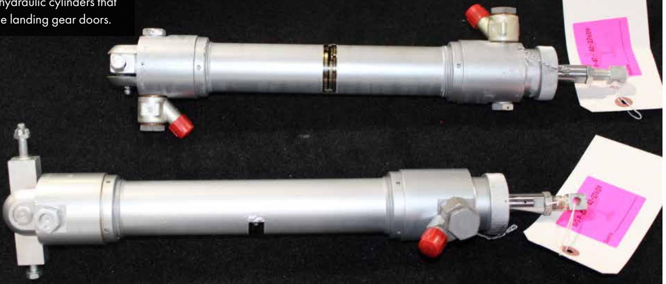
These are the wing flap operating cylinders.
