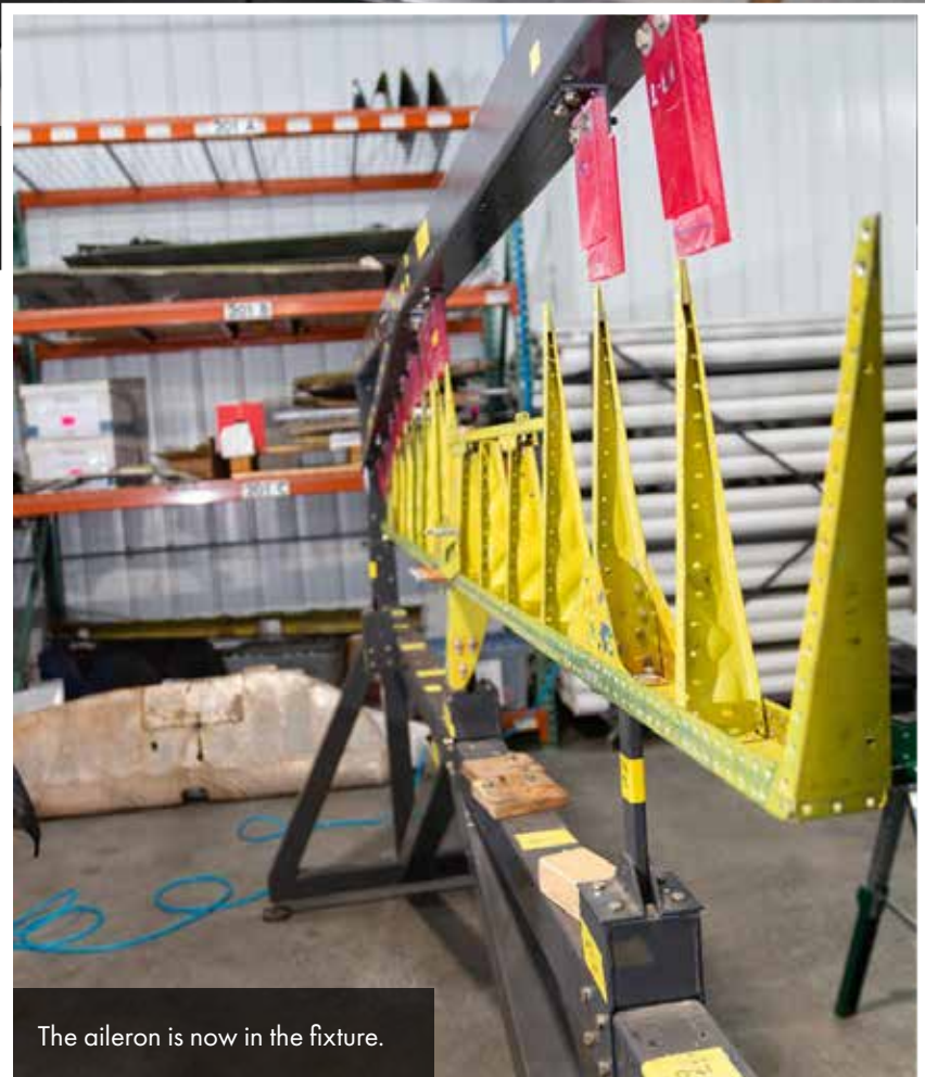
The aileron ribs have been installed to prepare the aileron for mounting in its assembly fixture.
