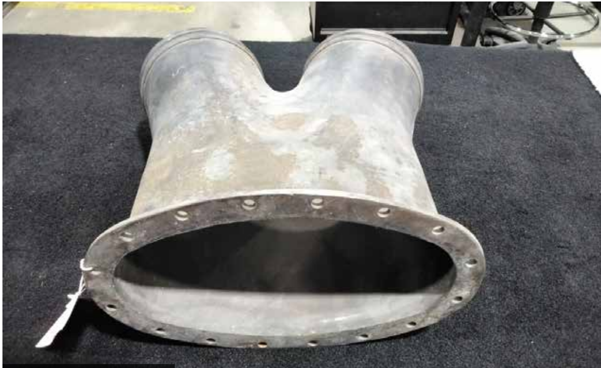
The single opening mates to the turbosupercharger inlet.
