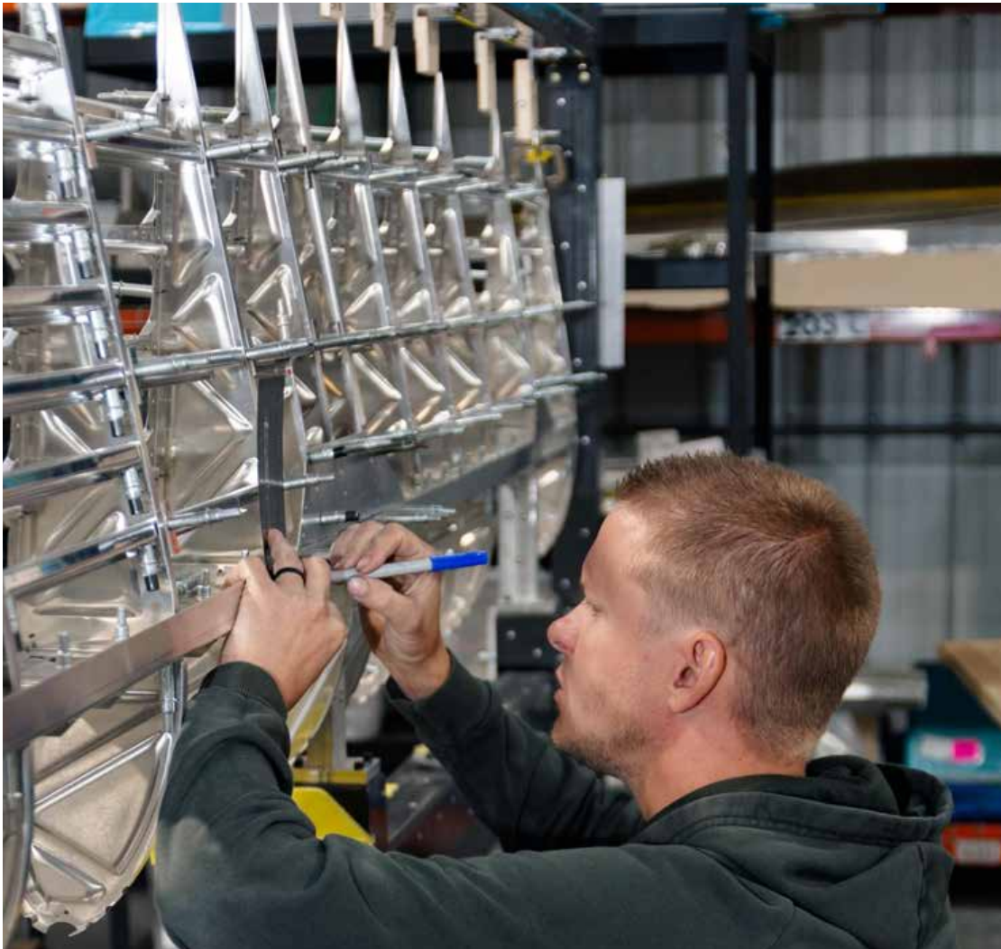
Many rivet holes must be located precisely and then drilled and deburred. Here Cory is marking the rivet spacing for the skins on the flap spar.
