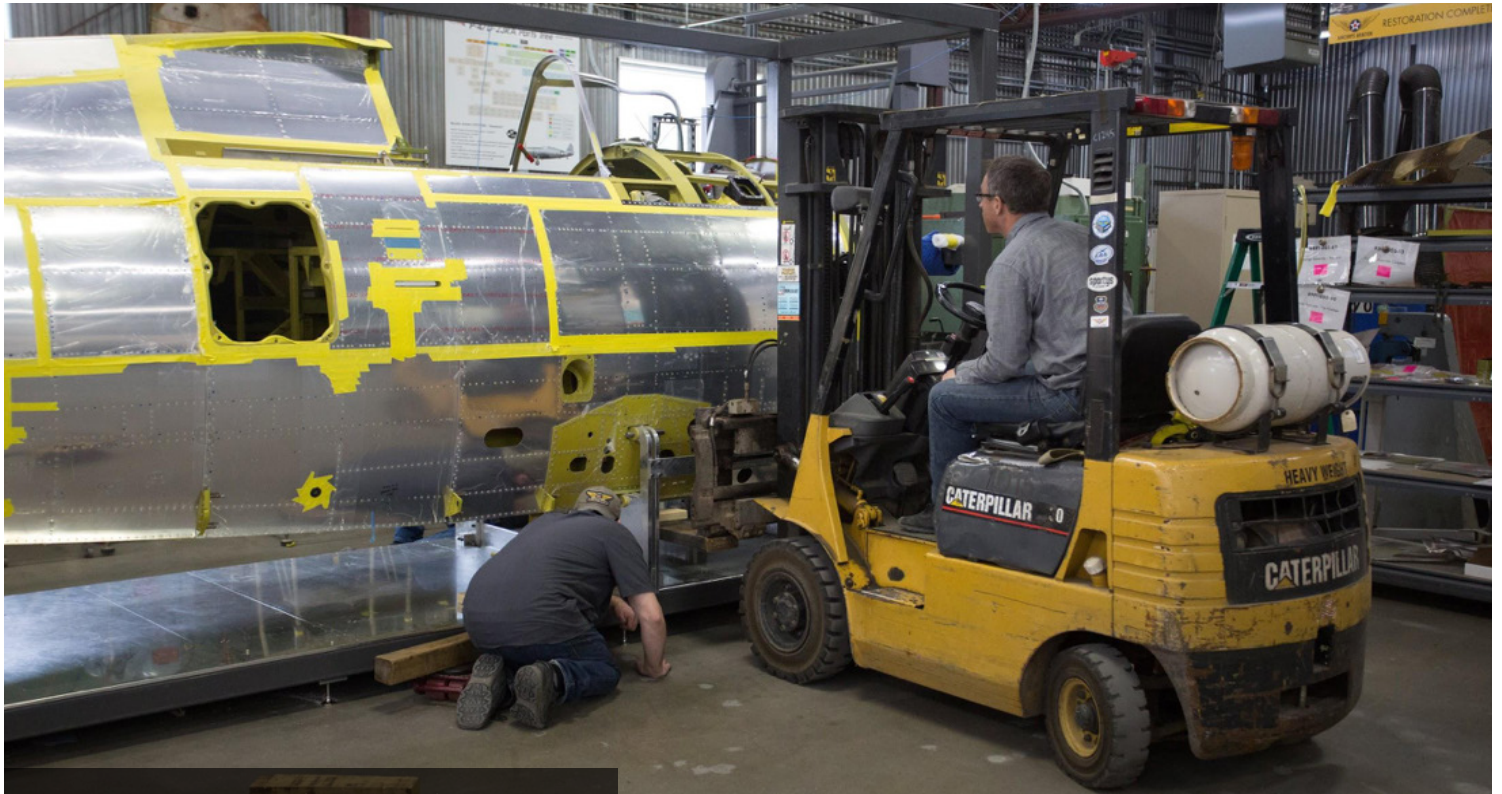
Randy is checking that the forks are perfectly aligned with the main fuselage longeron before lifting.
