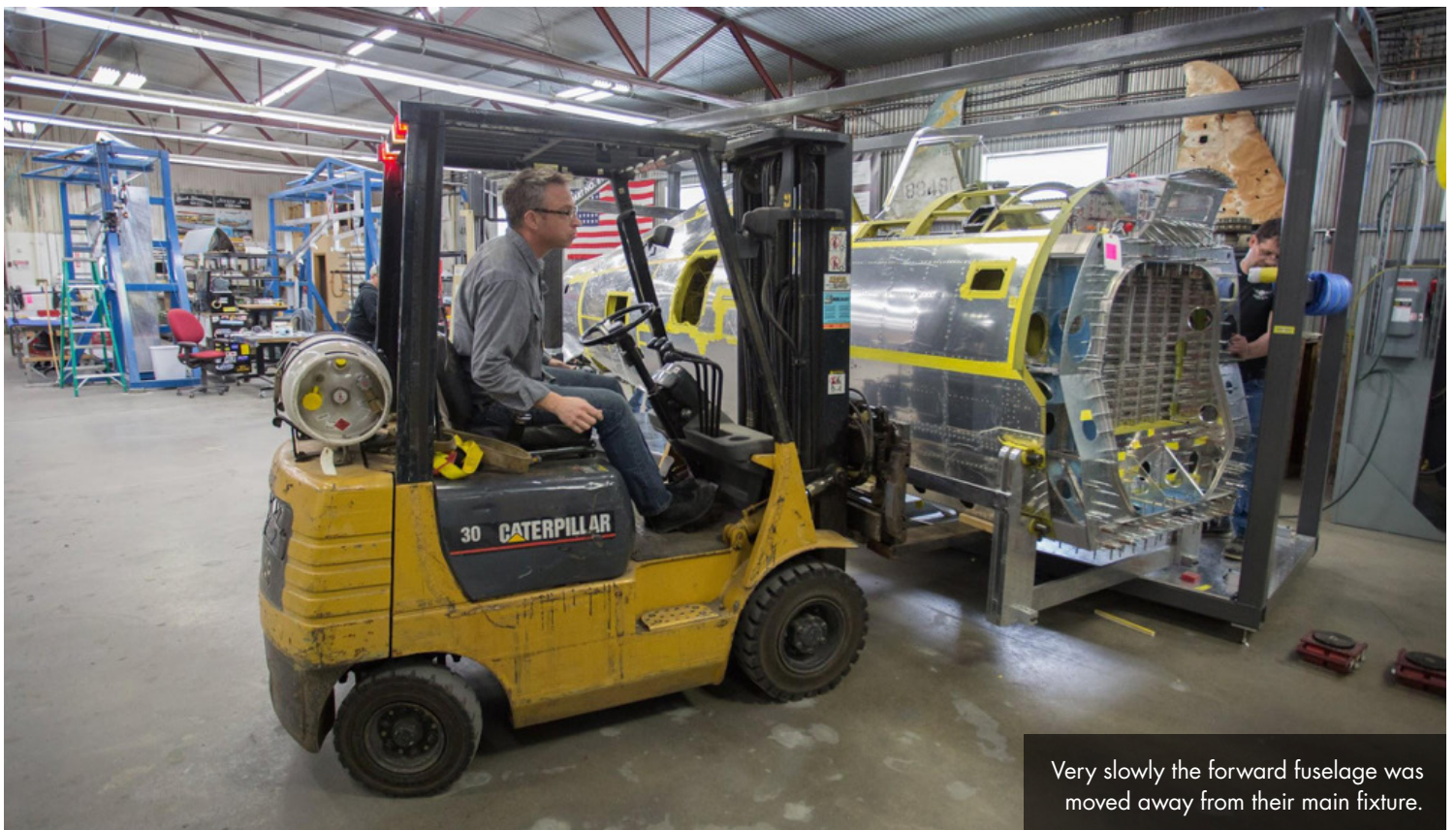
Randy is checking that the forks are perfectly aligned with the main fuselage longeron before lifting.
