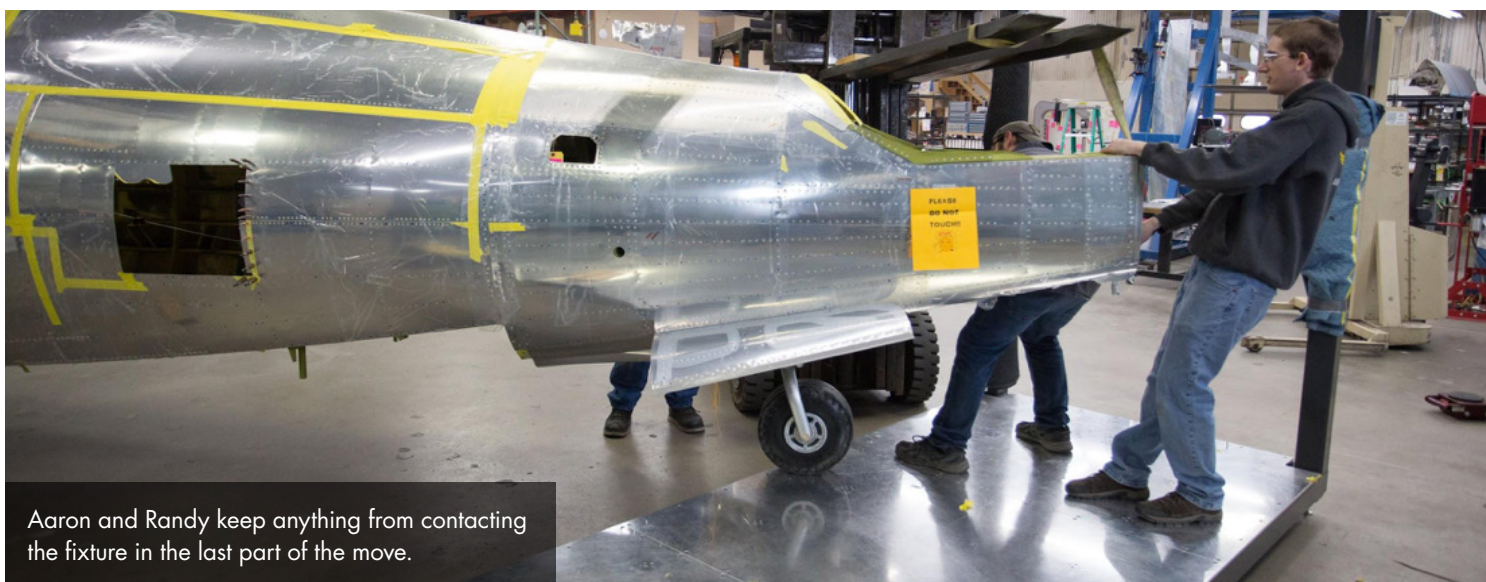
The move continues after the rear fuselage was set down on the tailwheel to reposition the straps.
