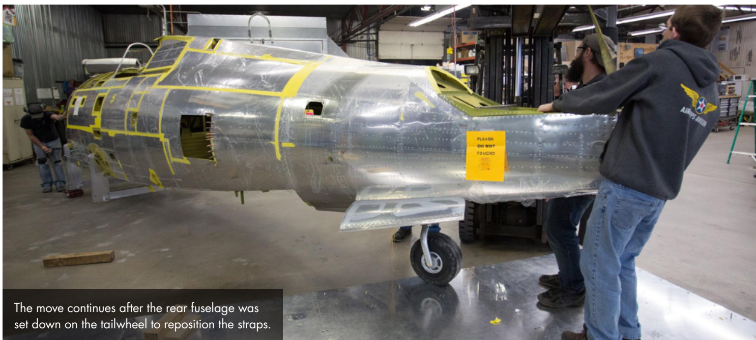
Next the fuselage was moved forward. The straps holding up the rear fuselage are just visible in this image.
