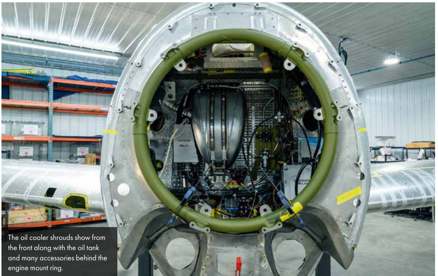
The larger openings on each side of the lower secondary cowl are shrouds for the oil coolers.
