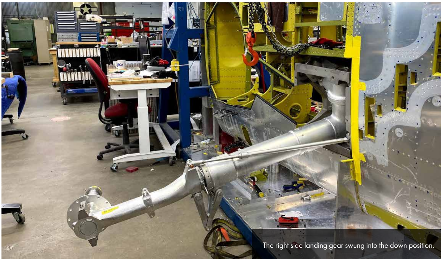
A big step in readying the wings for removal from the fixture is fitting the landing gear boxes.
