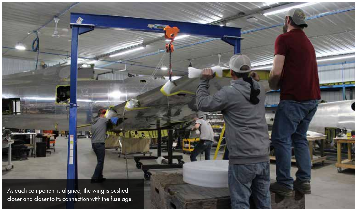
The holes in the wing attach fittings have to precisely line up.
