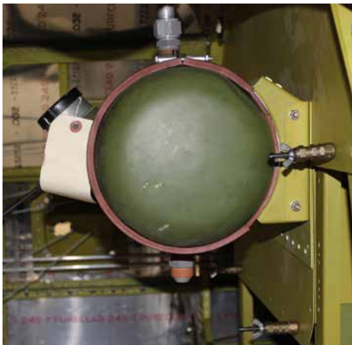
The supercharger oil tank is permanently mounted on the back of the Christmas tree tank enclosure.
