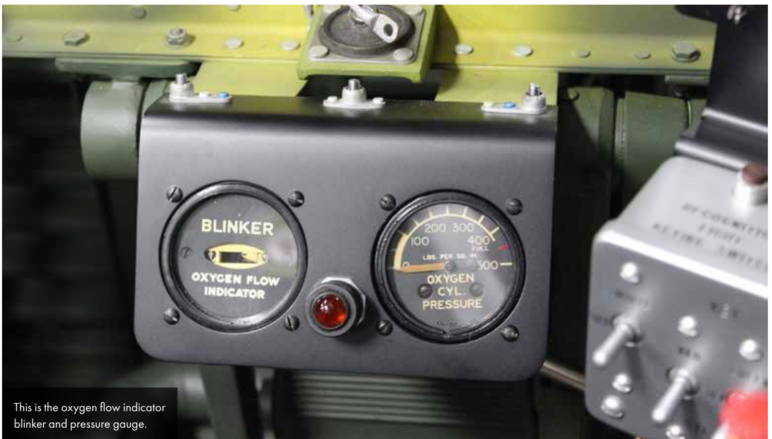
Systems installation continues, the upper black control subpanel has the primer and cowl flaps control, and attached below is the signal light box. The others will be identified in following detail shots.
