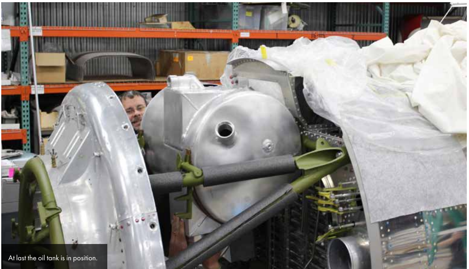
It took a lot of wiggling and adjusting to get the tank into the crowded accessory area.
