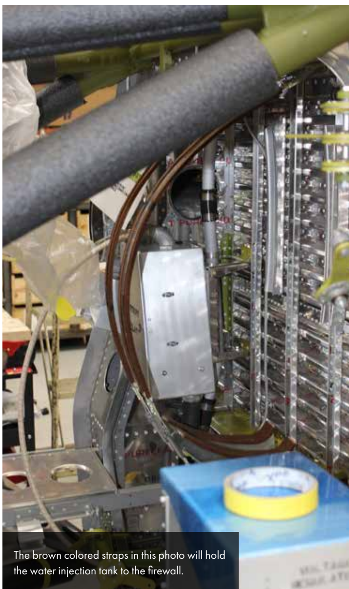
This closer image shows the metal straps cushioned by cork.
