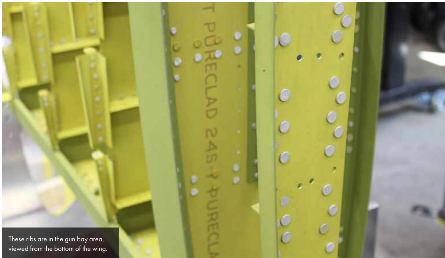
Progress in final assembly and riveting on the left wing is shown clearly in this shot.
