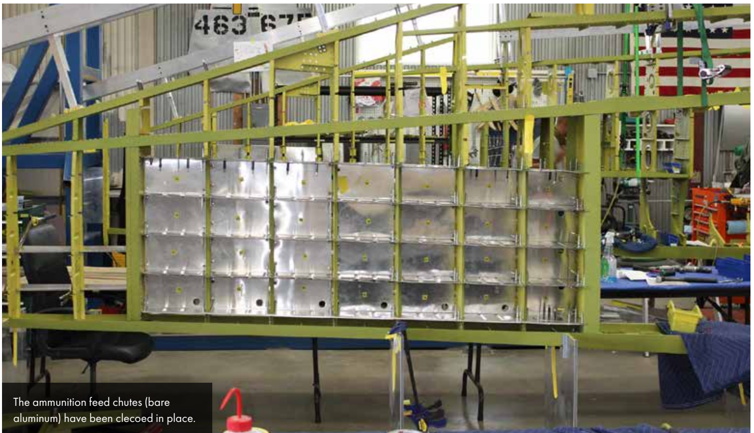
The right wing is shown with the gun bay ribs in place.
