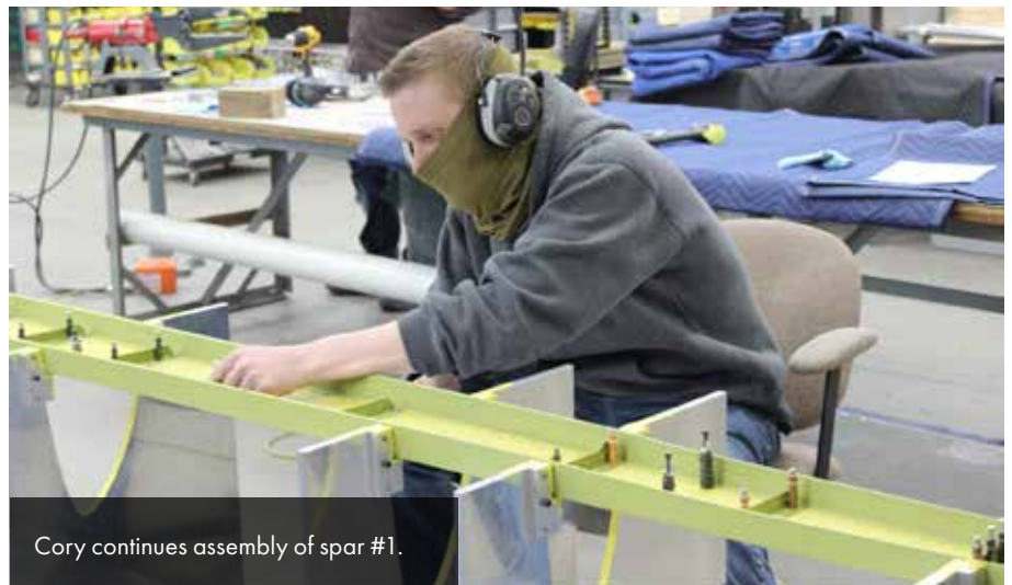
The fixture holds spar #1 as Cory works.
