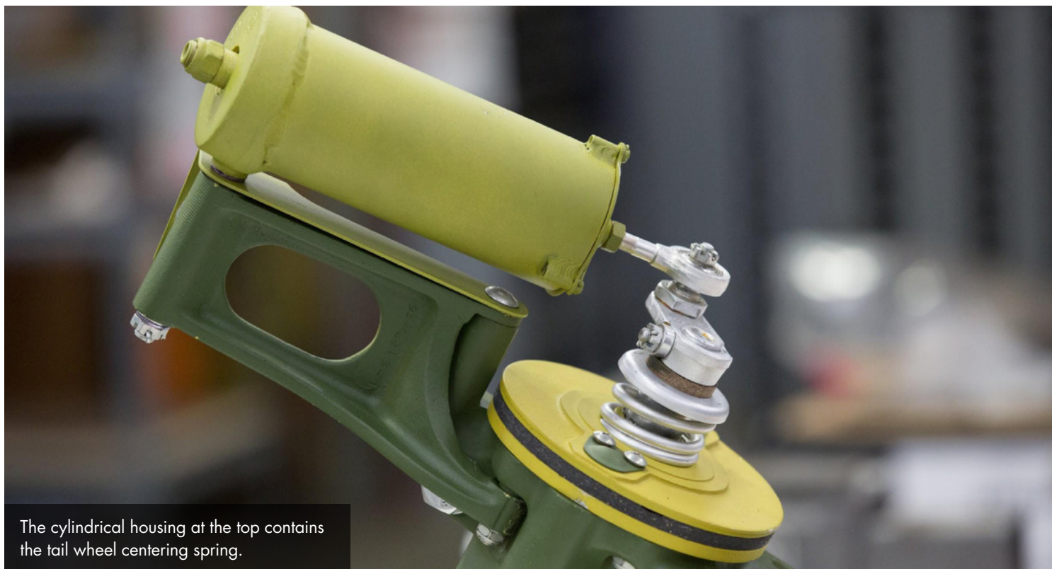
The tail wheel assembly is complete except for the actual wheel and tire.
