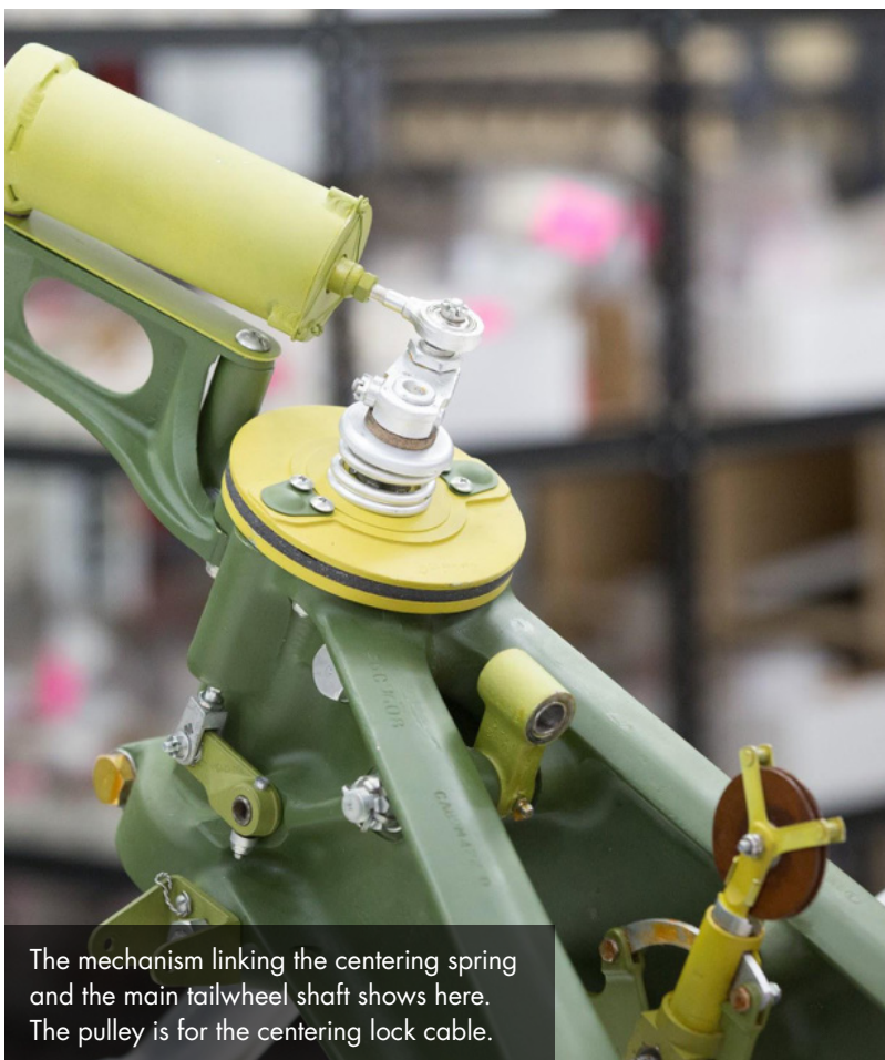
The linkage is the tail wheel centering lock.
