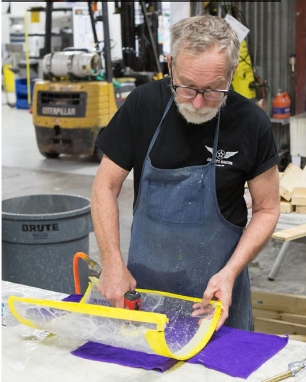
George has been working on creating the curved window panels for the cockpit enclosure.
