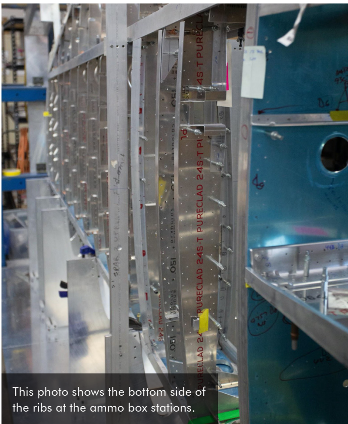
The rib sections with the curved ends facing the top of the image are shaped that way to accommodate the leading edge of the flaps.
