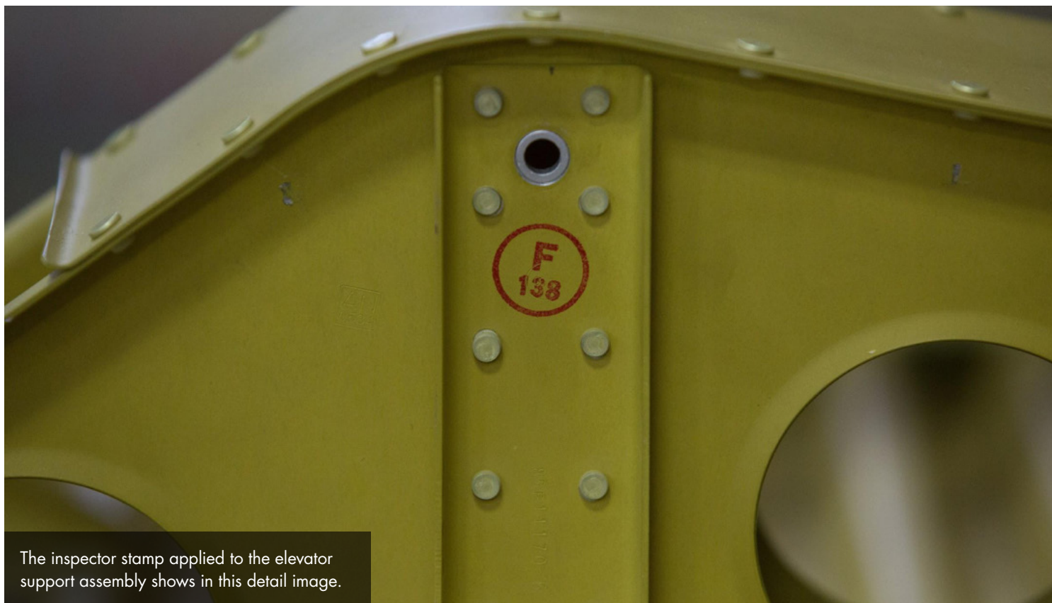
The elevator lever support has been painted and reinstalled permanently at stations 180- to 197.5
