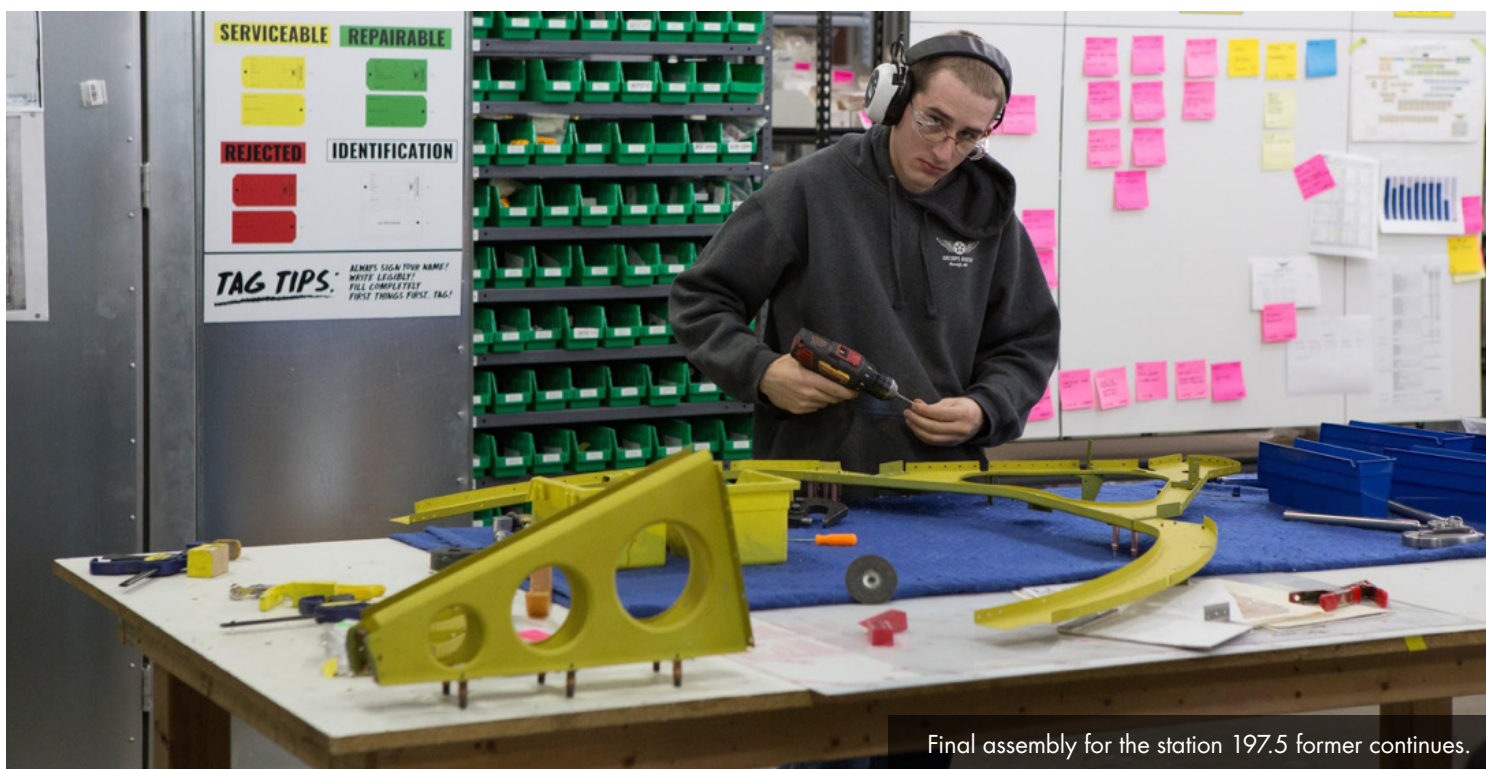
Aaron squeezes a rivet on a fuselage former. It will be the second fuselage former back from the cockpit, station 197.5.
