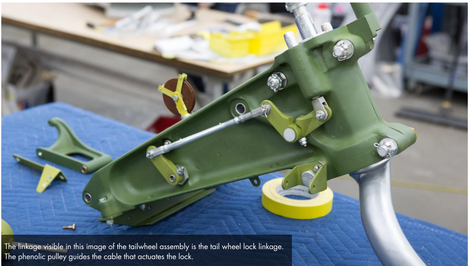
Tailwheel assembly parts are laid out on the bench. The large casting in the foreground is the tailwheel oleo strut brace
