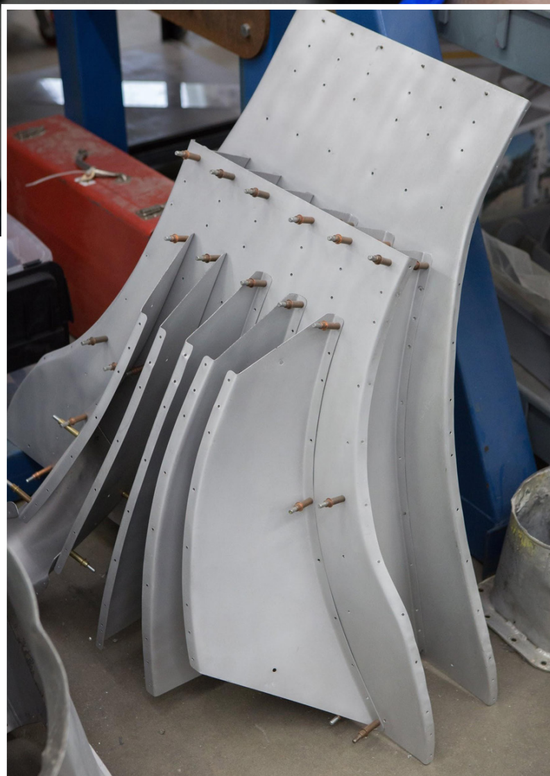
This interestingly shaped subassembly goes inside the carburetor intercooler air intake duct. It functions as an air separator to prevent turbulence in the airflow to the intercooler.
