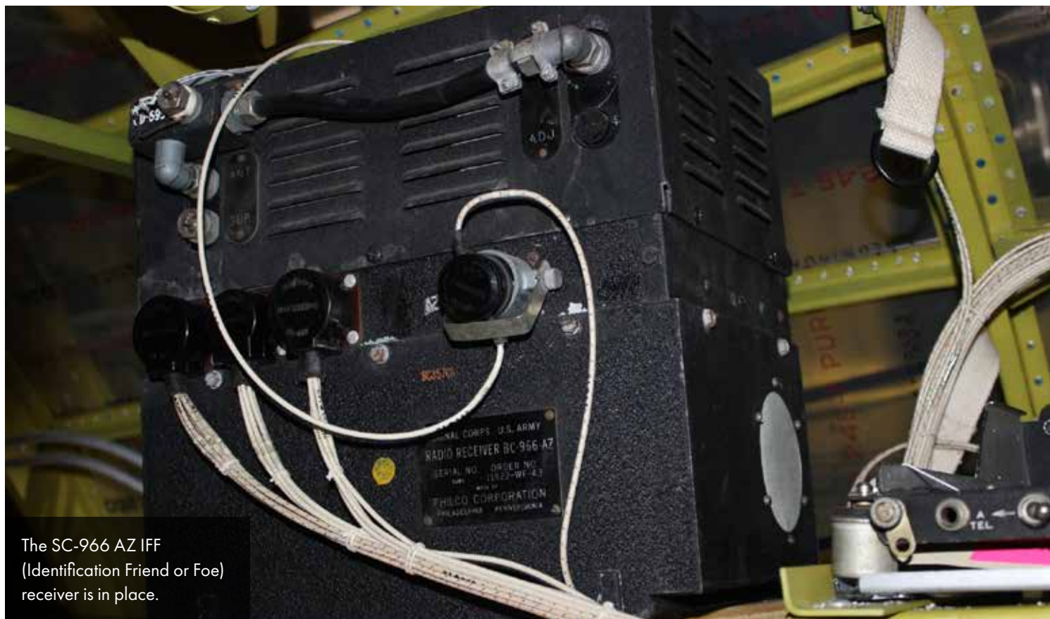
Aaron is using a spare receiver to test the fit of the non-stock mount that was necessitated by the 5th Air Force field modifications to accommodate the Christmas tree fuel tank.
