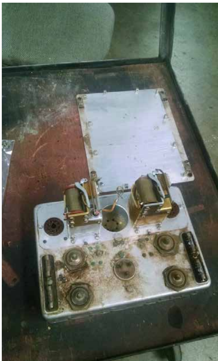
This is the modulator before restoration, John Castorina photo
