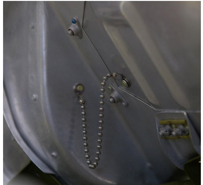
The small bead chain allows ground crewman to let the access door hang open once it was unbolted, without fear of it dropping to the ground or being misplaced.
