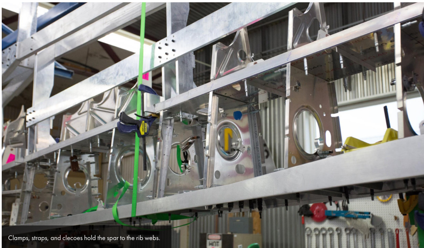
Visible in this shot are the station points that will fix the leading edge in place as they are added.
