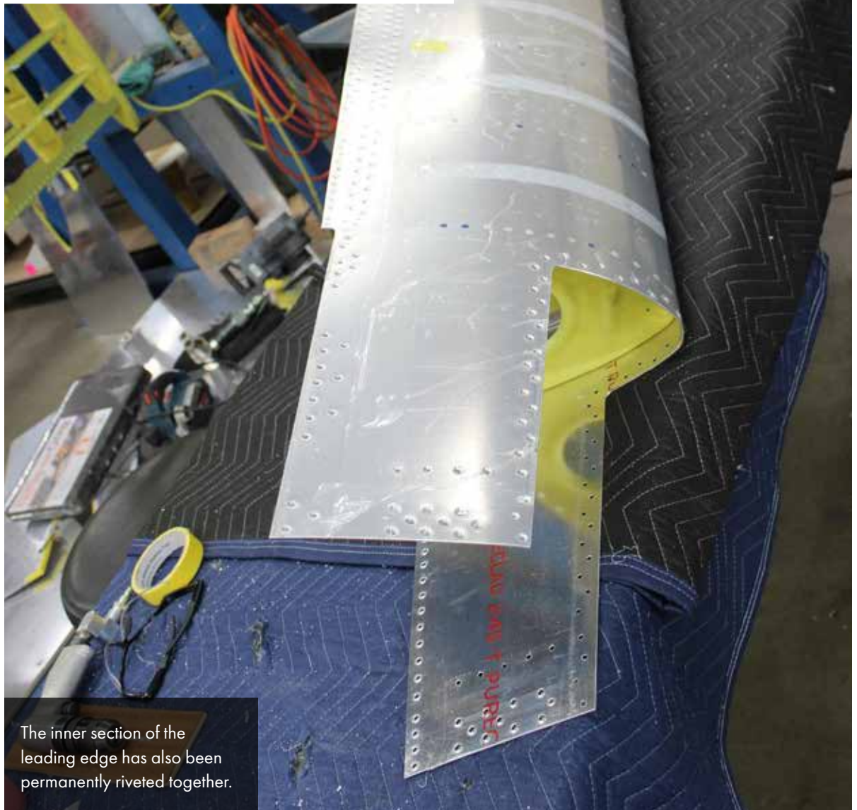
This angle shows the internal structure of the outer leading edge.
