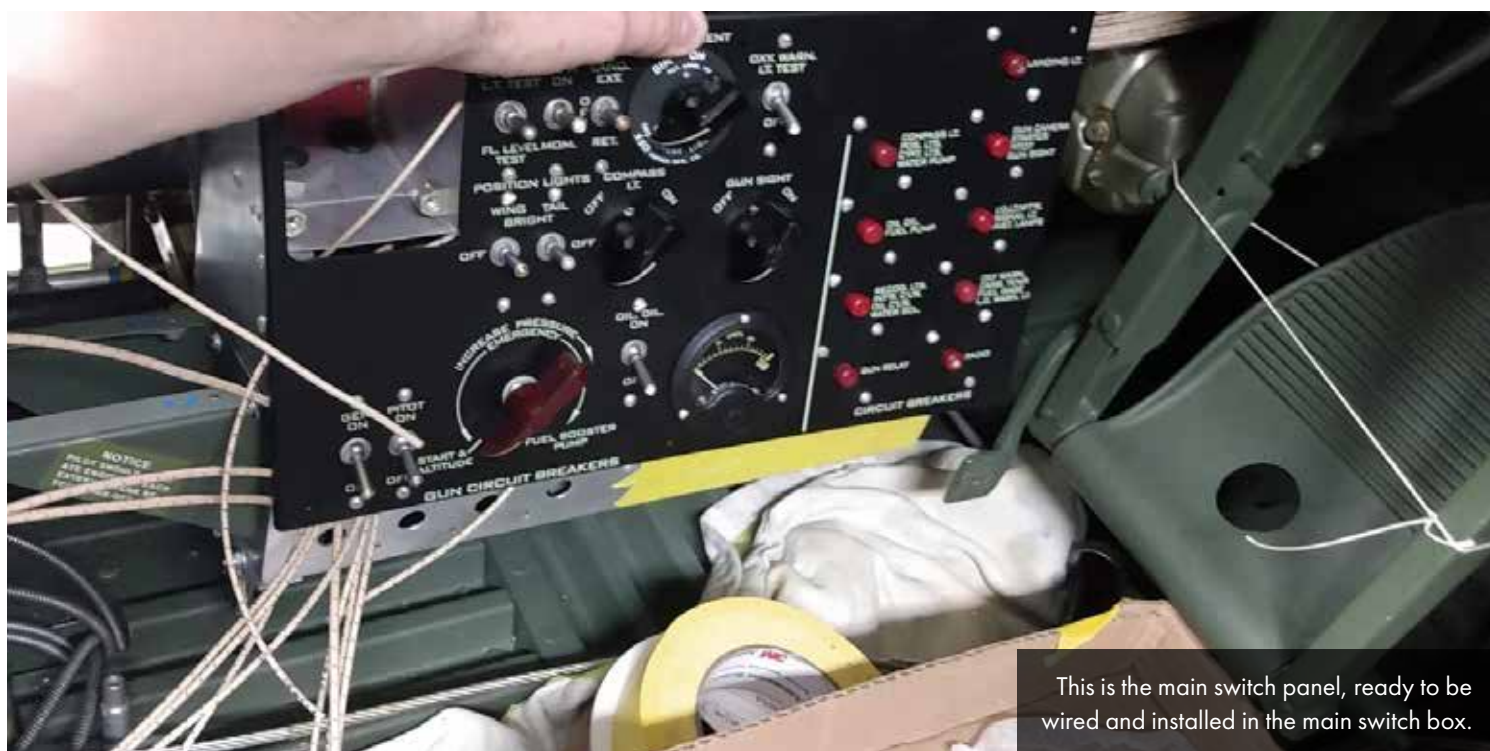
The main switch box with all the wires led into it is ready for the switch panel.
