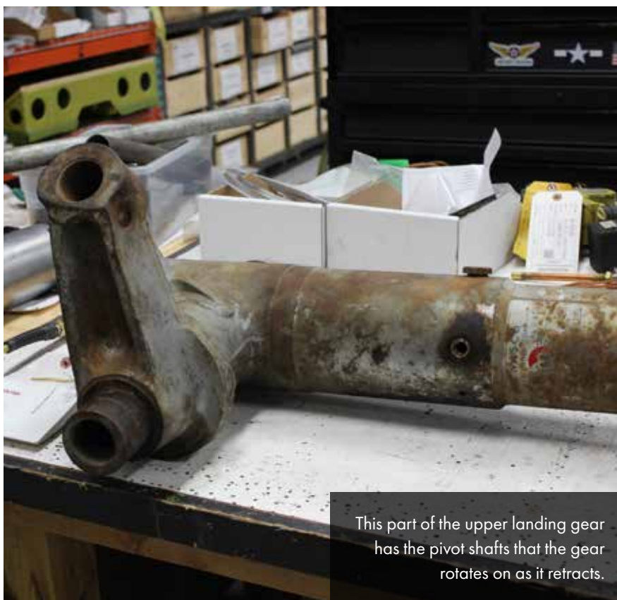
The P-47 main landing gear strut is almost as long as this eight foot table.
