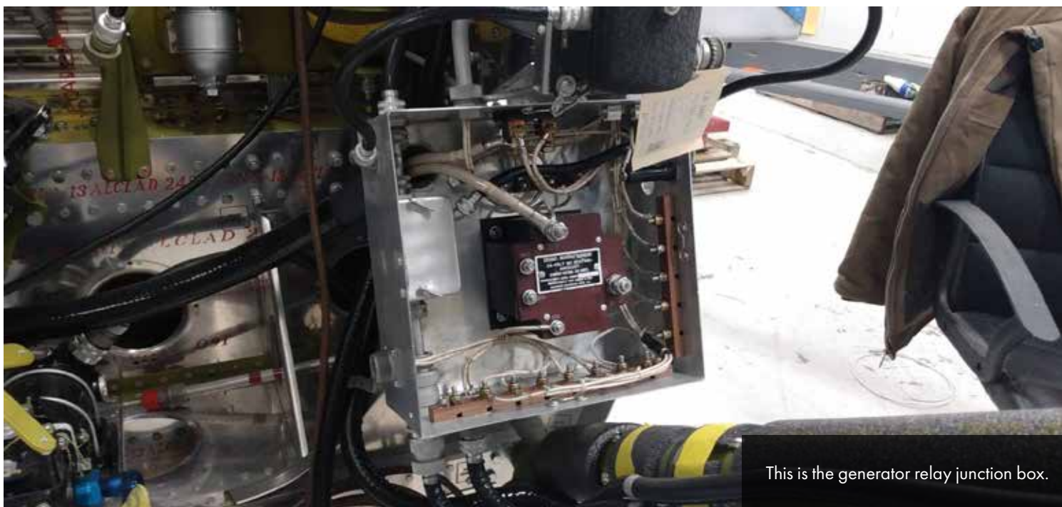
This relay box is for the Curtiss Electric prop.
