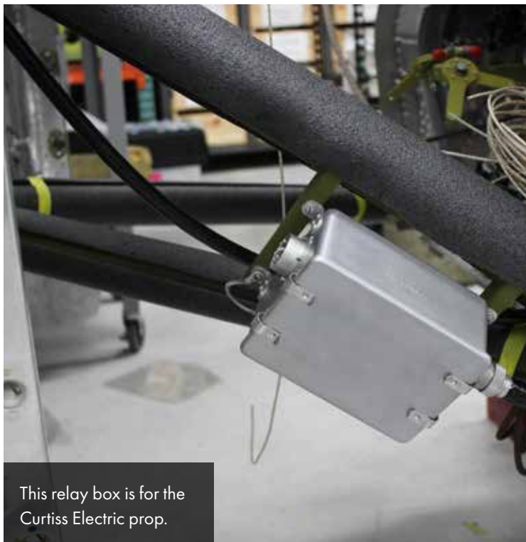
The ground power unit plugs into this receptacle.
