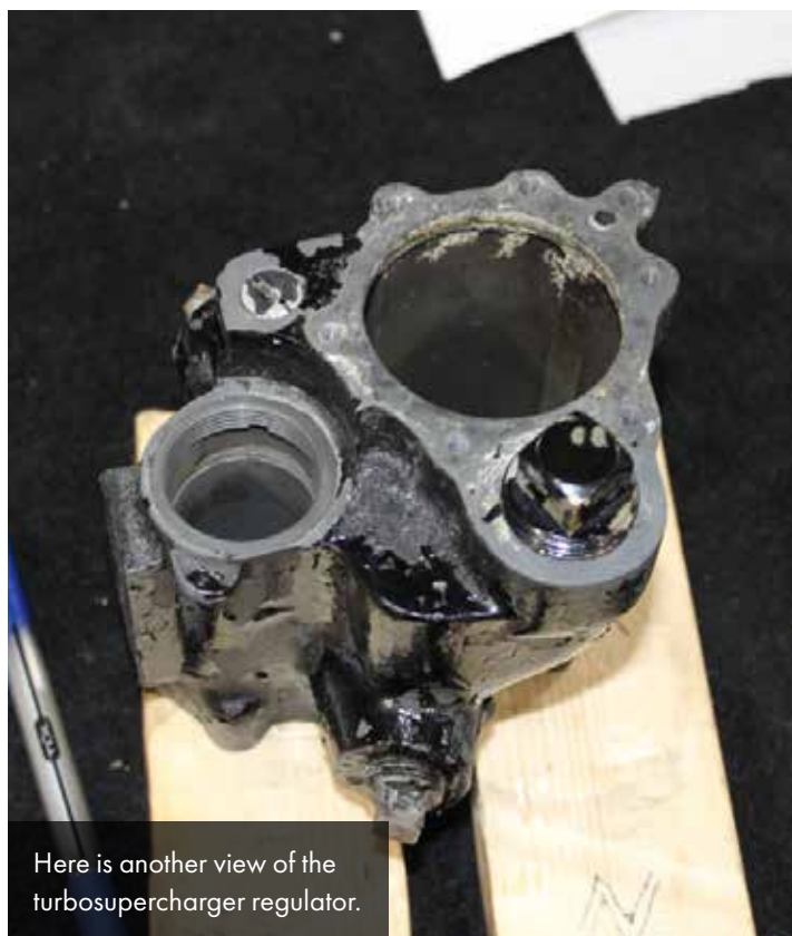
The turbosupercharger regulator regulates oil pressure to operate wastegates.
