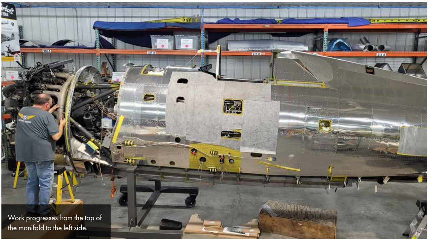
Mark works on assembling the exhaust manifold.
