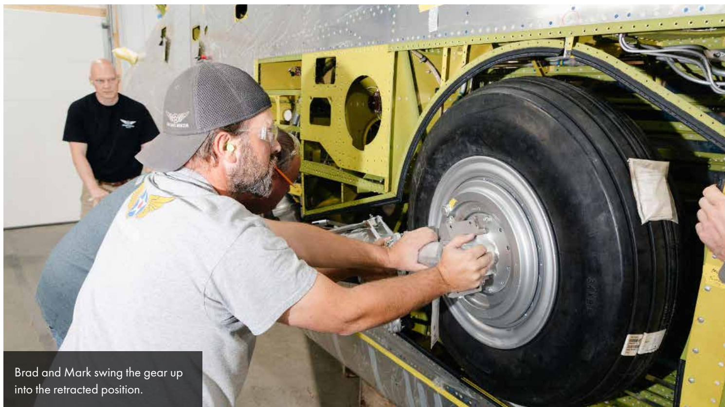
Mark and Brad work on the free movement on the left main gear.
