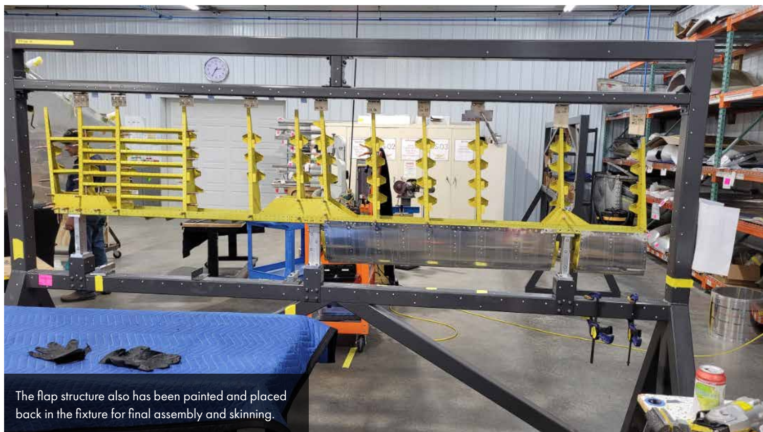
Work on skinning the rudder continues after the internal structure has come back from the paint shop.
