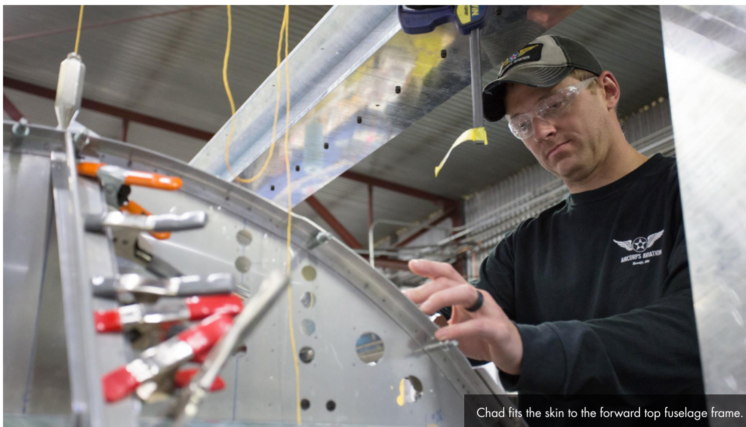
Chad works on a piece of skin located on the upper fuselage in front of the cockpit.
