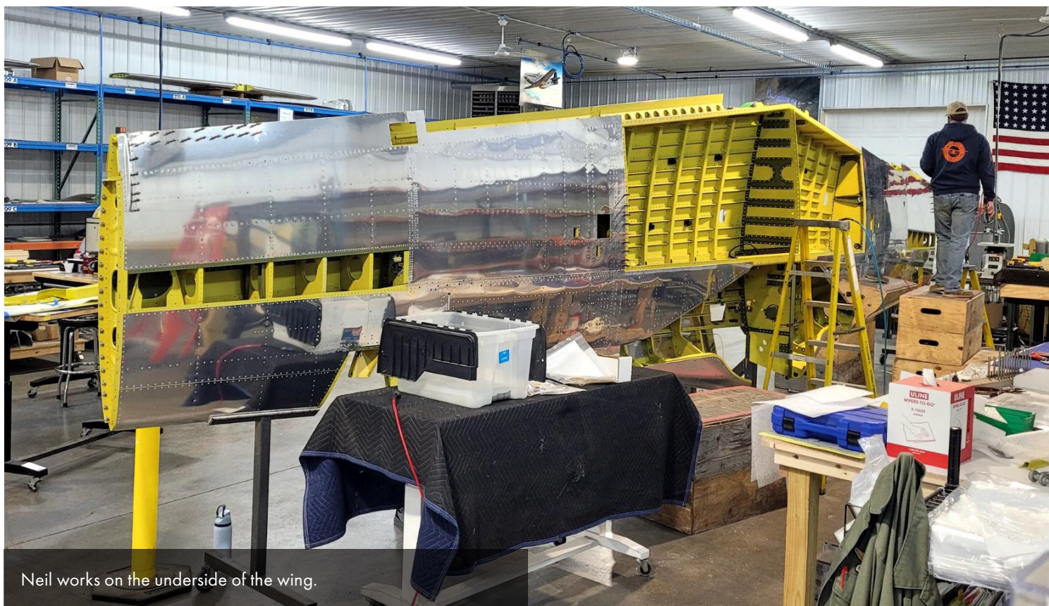
The wing is out of the fixture and mounted on rolling dollies. The fixture used for the construction is visible behind the wing.
