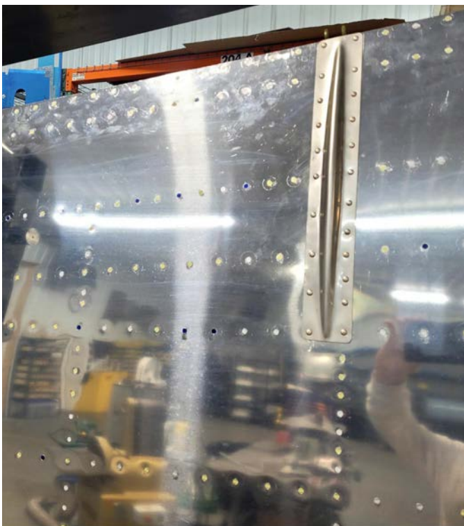
Stiffeners have been added to both wings, just inboard of the wing extensions.
