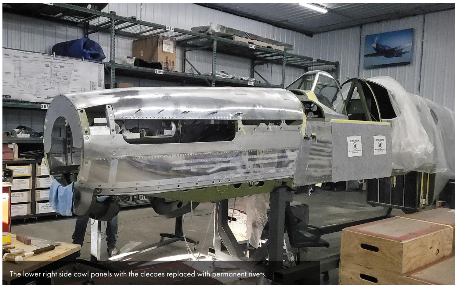
The lower cowl panel is clecoed on for fitting.
