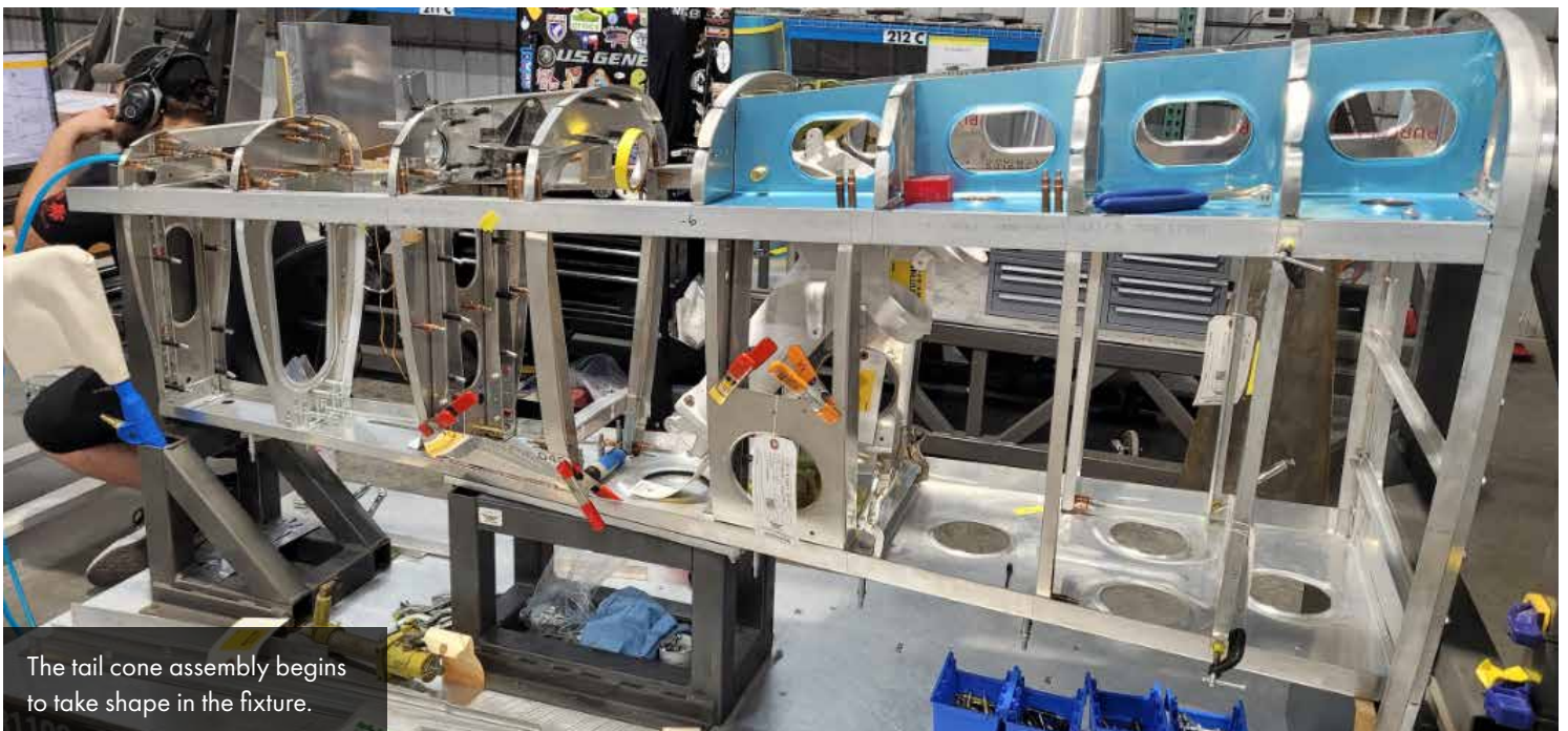
The first fuselage formers are in place in the fixture.
