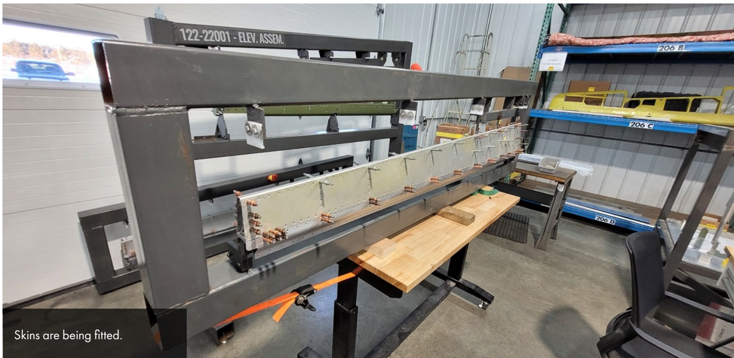
Once the aileron structure has been assembled, it goes to paint and subsequently returns to the fixture for skinning.
