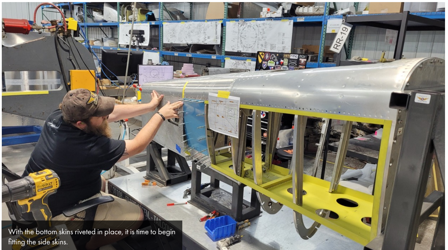
The bottom skin has now been riveted in place.
