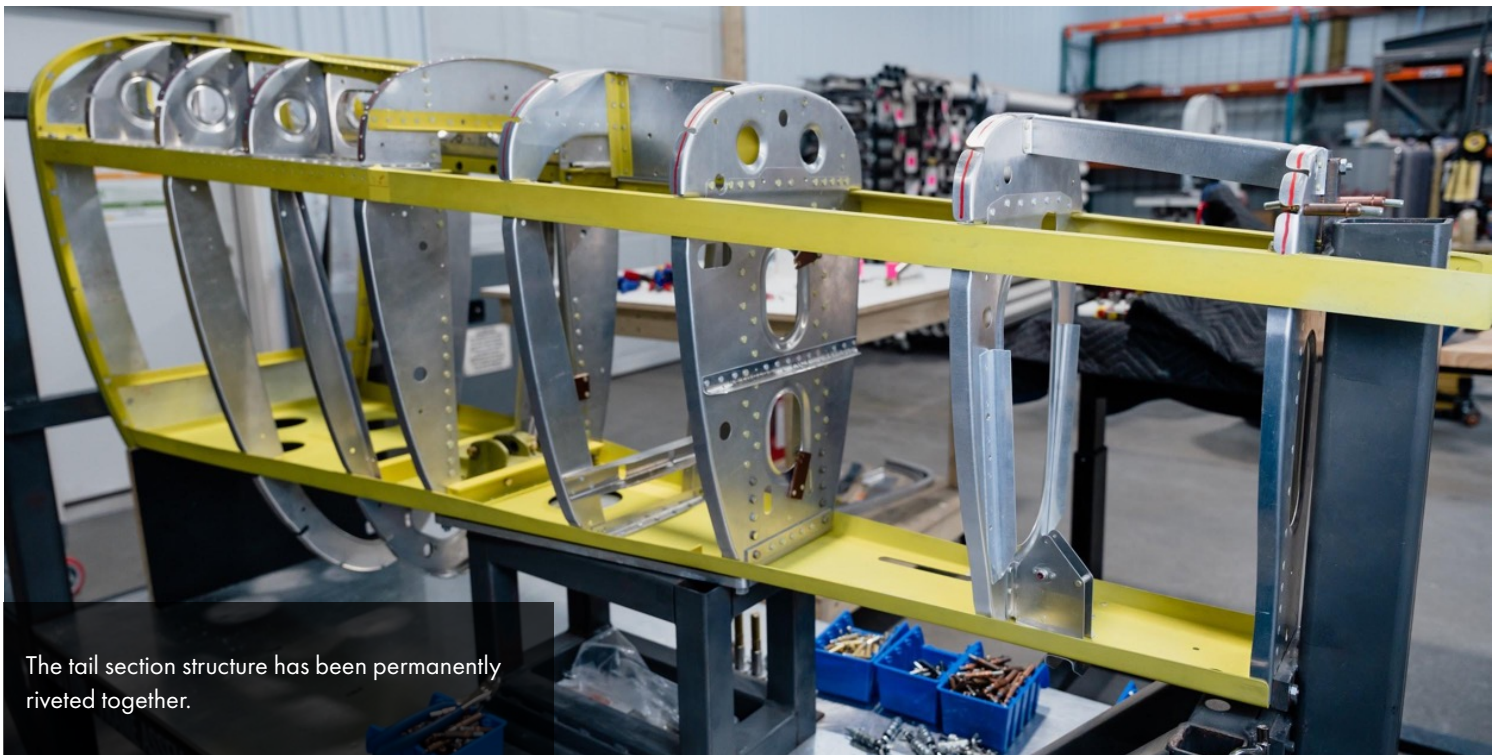
Back at the restoration shop after painting, the tail cone assembly has been returned to the fixture for riveting.
