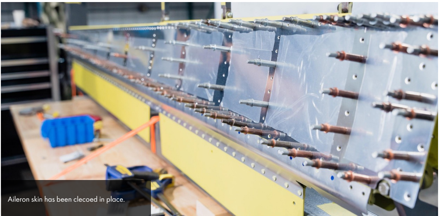
As the aileron takes shape, the part known as the aileron diaphragm is added (yellow piece on the bottom of the assembly). This part prevents drag-inducing air flow by closing any gap between the aileron and the wing itself.
