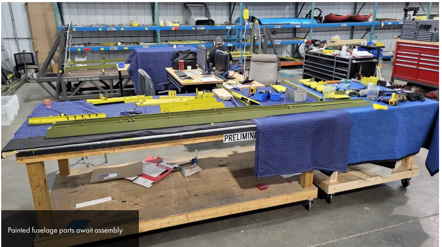
The fuselage components have been painted and returned to the restoration shop. Brad begins the process of permanent assembly.
