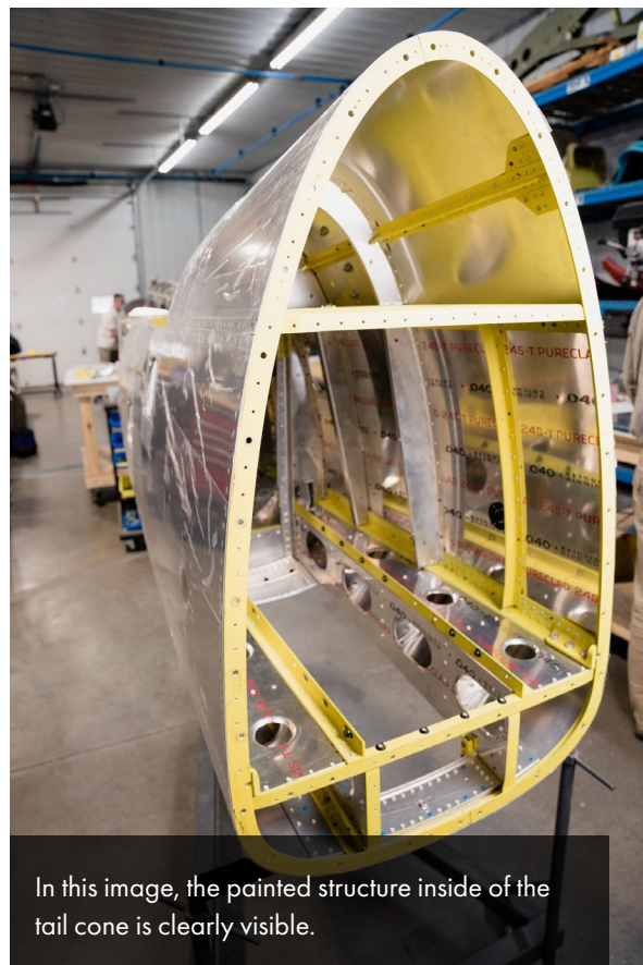
This bulkhead is just in front of the horizontal stabilizer opening. The two oval openings with brown phenolic parts riveted to them are for the upper elevator cables.
