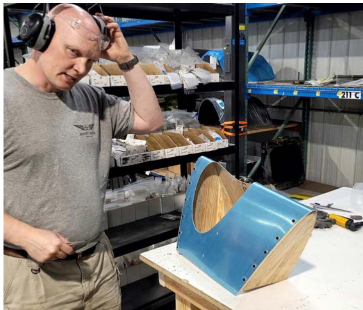
Jacob is fabricating and forming the leading edge skin with the landing light opening. The P-51A, B, and C Mustangs had this type of landing light in the left wing leading edge. The A-36 Mustang had a slightly wider opening to accommodate two landing lights, and the later D models had retracting landing lights located in the wheel well.
