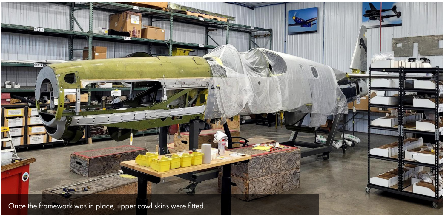
As work began on the firewall forward section, the cowl support formers were installed.
