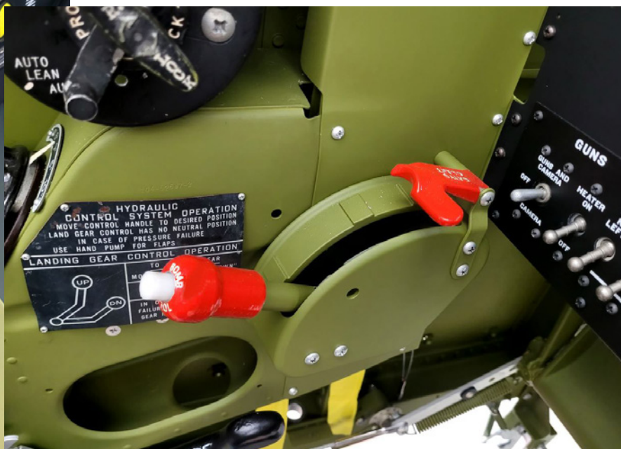
The bomb control sector mounts on the lower left cockpit side near the bottom of the instrument panel. The gun switches are on the panel seen in the center right edge of the photo.
