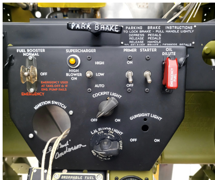
The pilot's main switch panel is installed and awaits the ignition switch wiring and installation.
