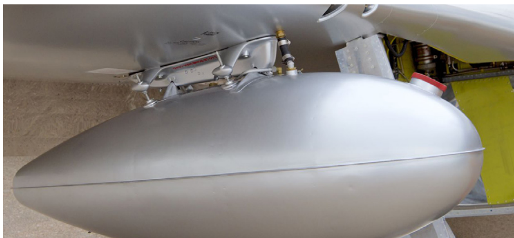
A historically accurate all-cast B/C model bomb release on Lope's Hope 3rd. Photo by Scott Slocum from Lope's Hope 3rd judging book.
