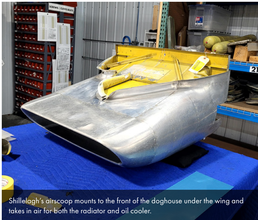
Potential components of the carburetor air induction system are organized on a table for inspection as the time for their fitting and installation nears.
