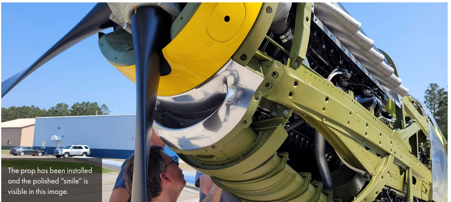
There's more fitting work for Mike as the upper nose skin is finished.
