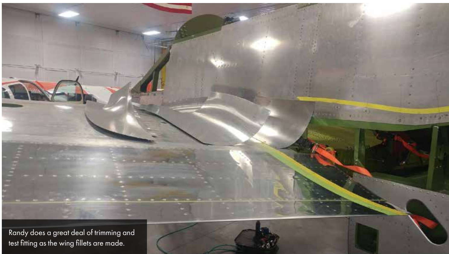
This closer image accents the complex curves at the rear of the wing fillet.
