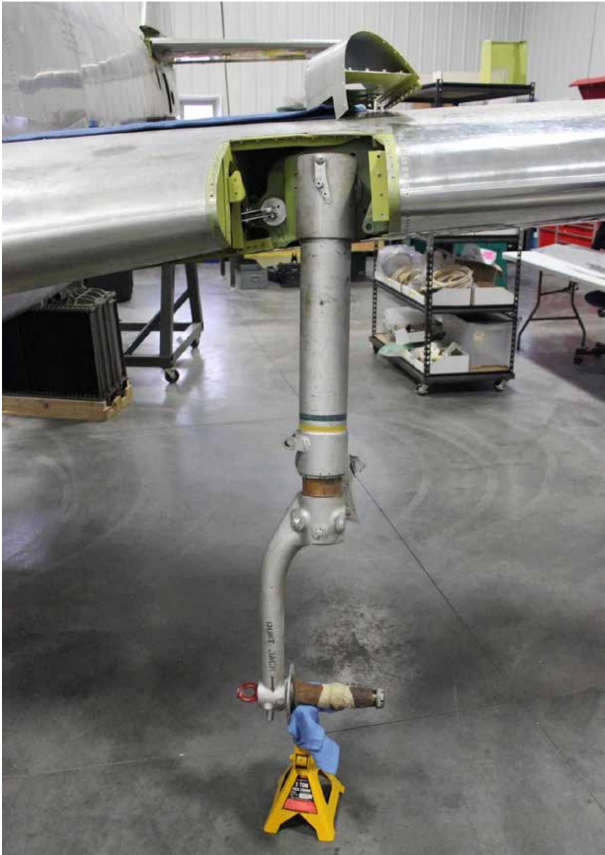
Thunderbird's landing gear is original to WWII, and has never been installed on an aircraft until now.
