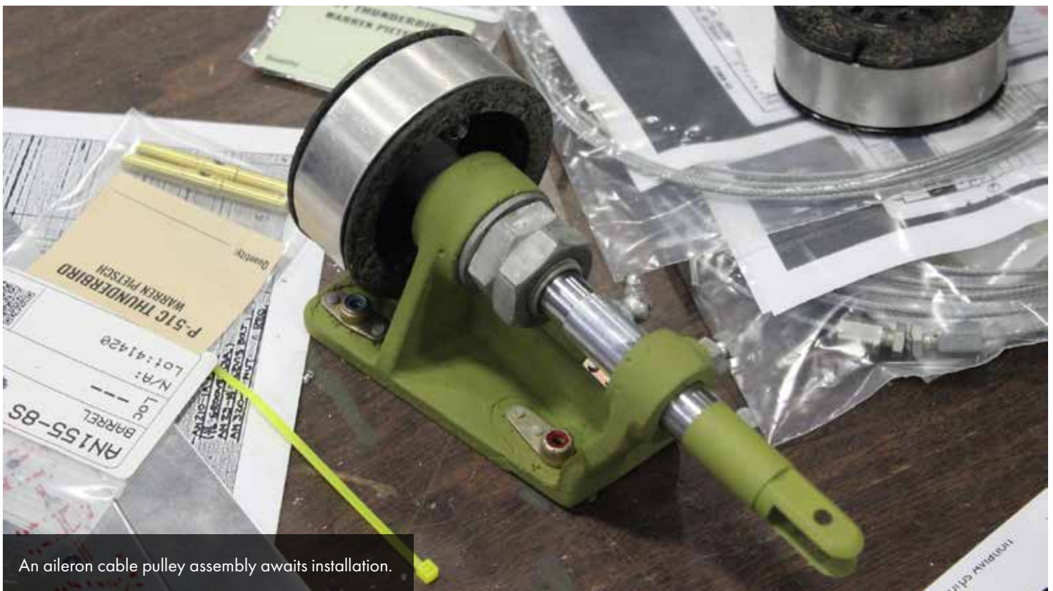
Aileron cable subassembly parts sit on a bench with the control stick torque tube they'll eventually be connected to.
