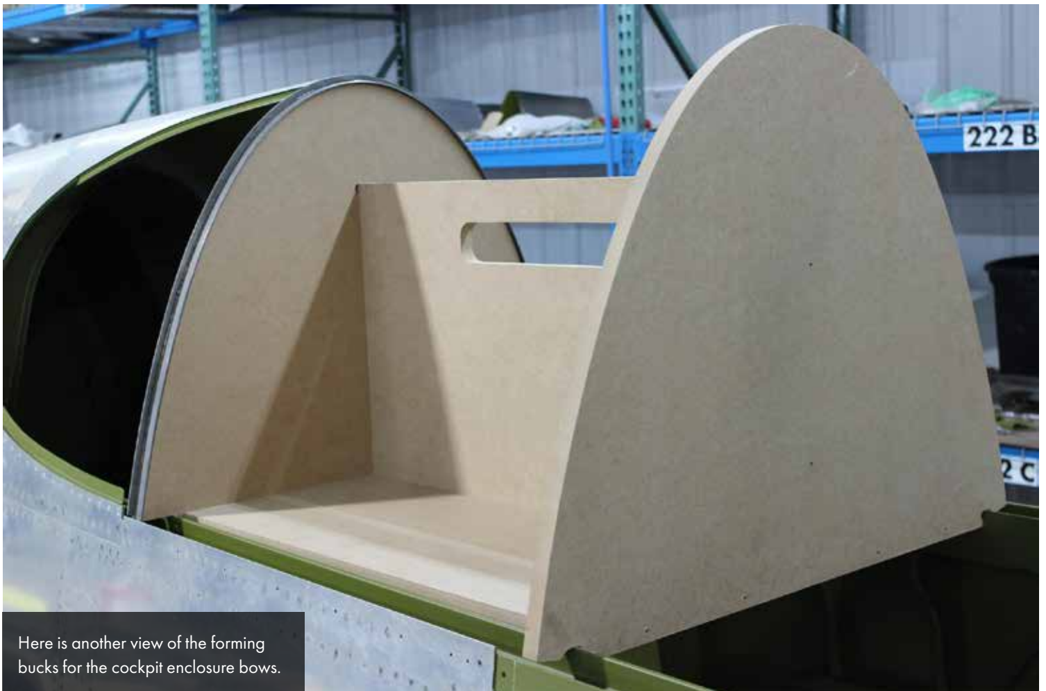
MDF particle board bucks have been installed to help form and fit the cockpit enclosure bows.
